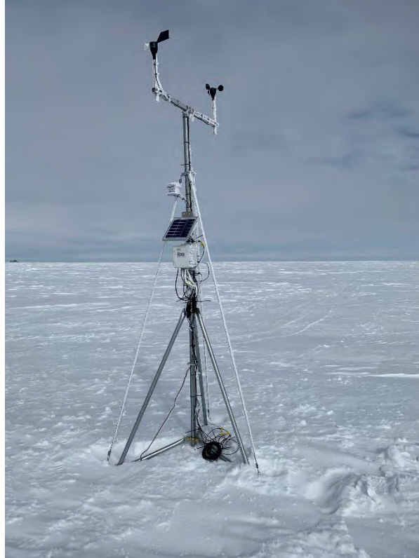
Figure 6. Meteorological (MET) station deployed on the sea ice in our study area. Data were downloaded from the MET station onto a laptop computer weekly.
