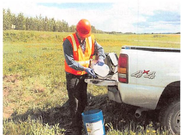
DEC's Dennis Shepard is shown decontaminating a water interface probe during a groundwater monitoring well
