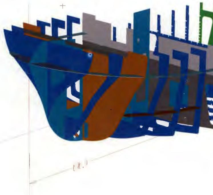
3. shown here are both sides of the anchor roller structure (in red), which are 6" apart, and solidly welded to the center longitudinal or bow stem.
