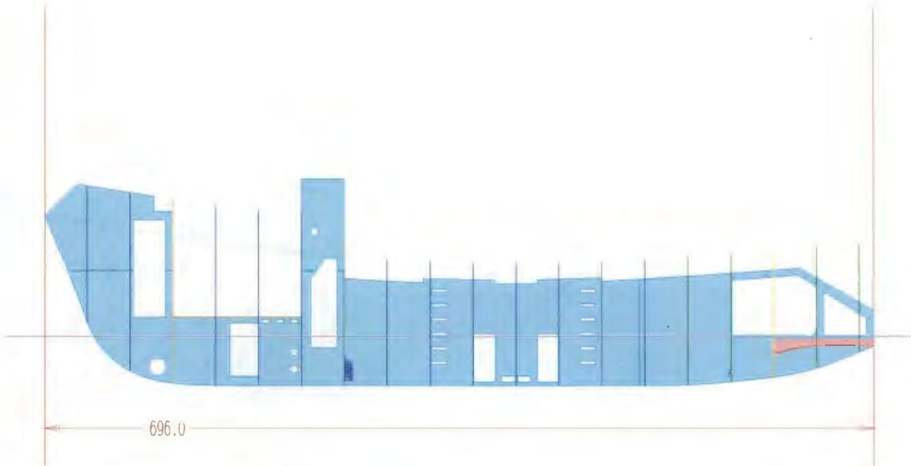
2 This view shows the center longitudinal (and bow stem) again, with the addition of the frames on 36" centers.
