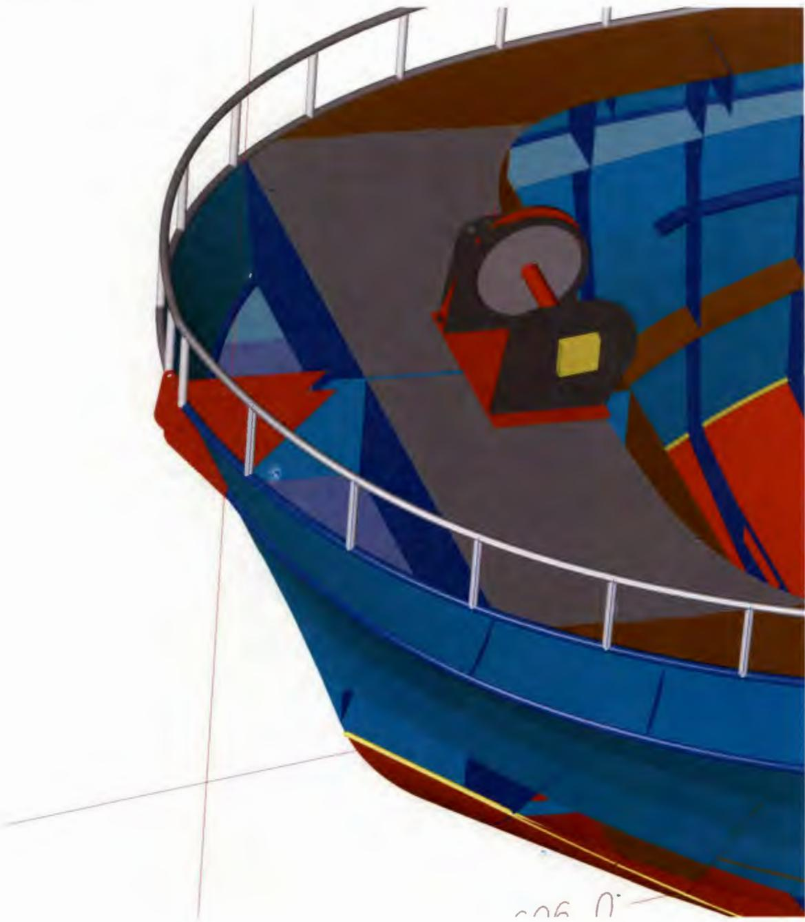
5. hull plating and forward bulwarks are wrapped around the frames and solidly welded into the bow roller and bow stem creating a buoyant envelope that is still 58' long.
