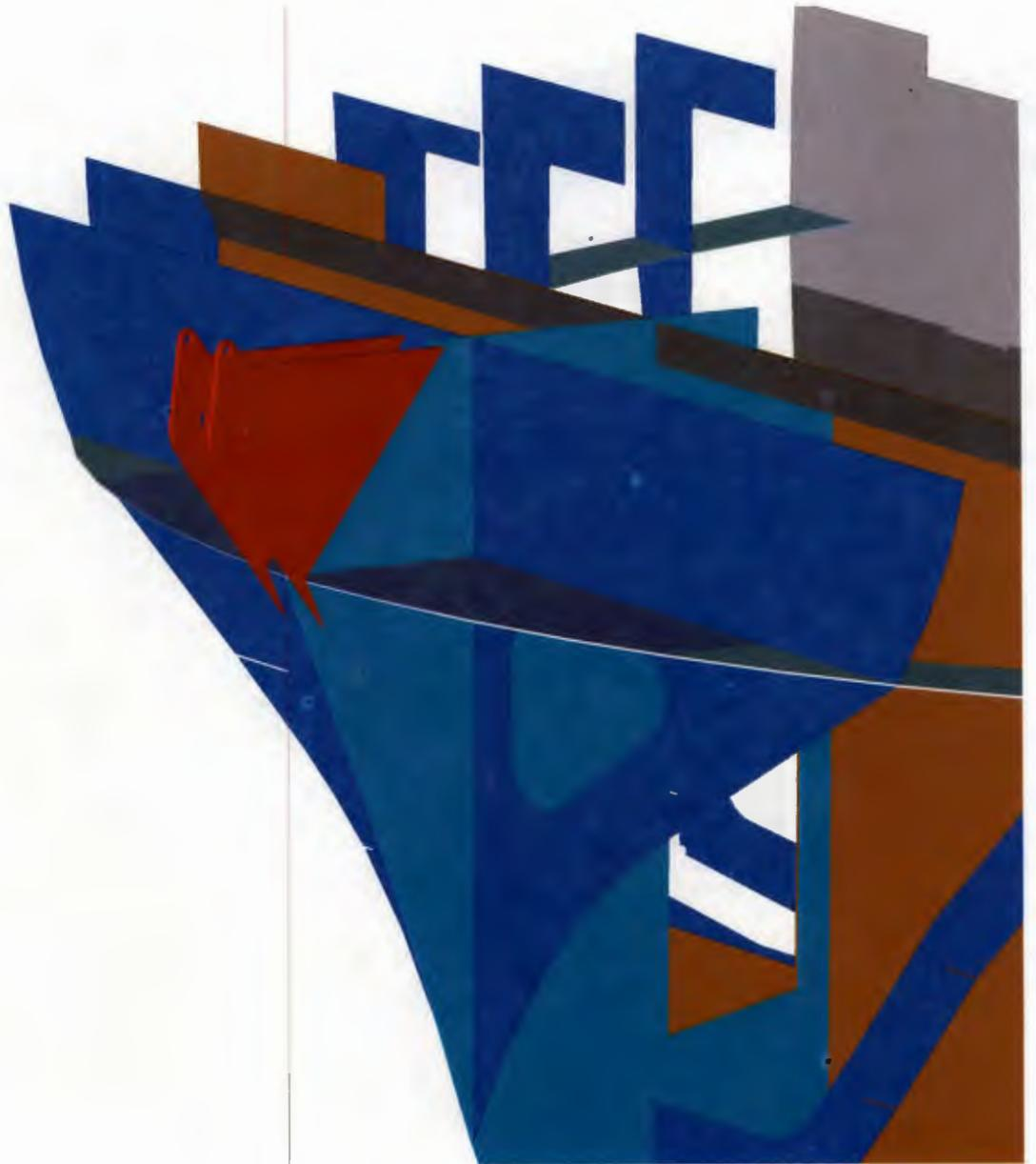
4. Deck plating (gray color) is added behind station 1 as roof to accommodate the needed head room in the below deck sleeping quarters.
