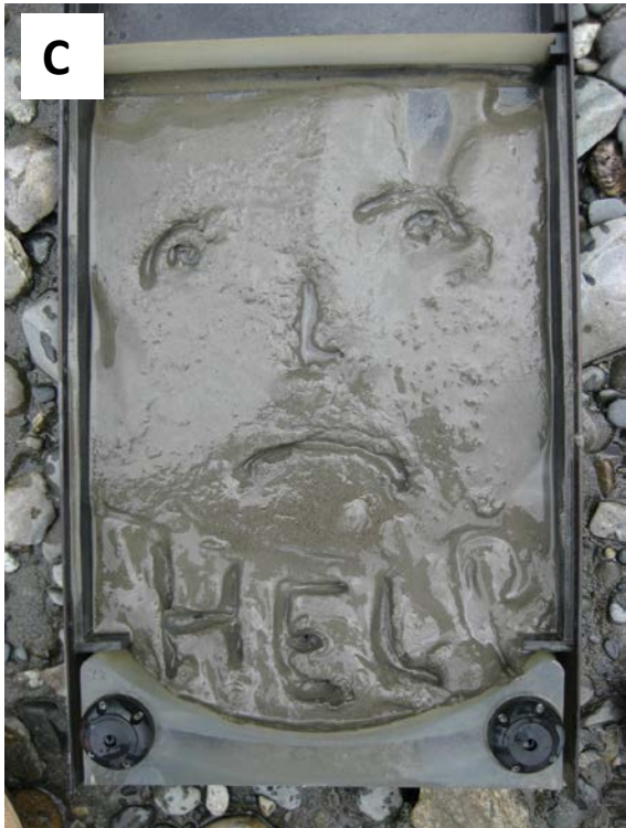
Figure 11.—DIDSON-LR with a high-resolution lens (on left in photos A and B) mounted next to a split-beam transducer (on right in photos A and B). A custom fit fabric enclosure shown in photo B protects against silt buildup in front of the lens as shown in photo C.
