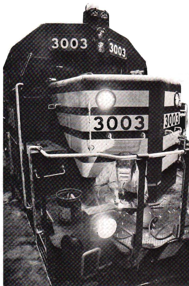
Frank Box, boilermaker for the Alaska Railroad, welds one of two lights that were attached to the locomotives to chase moose off the tracks.
