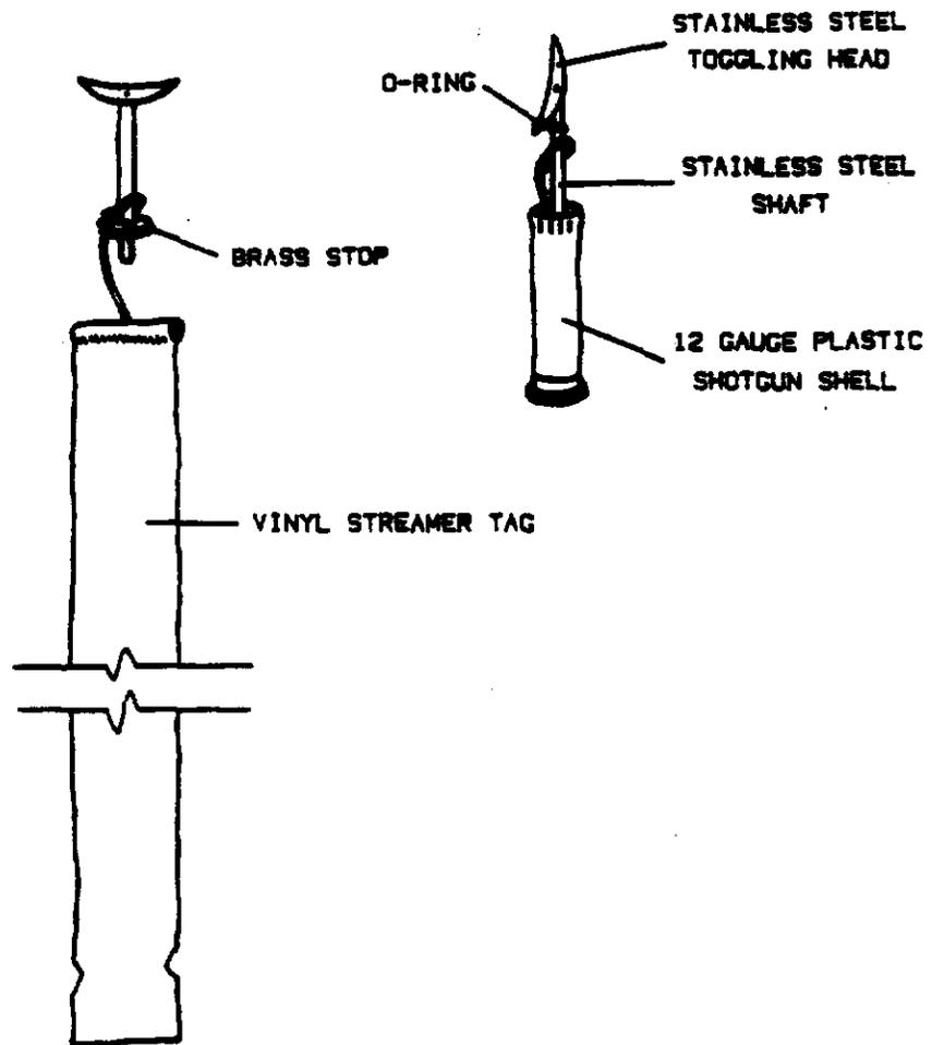
Figure 3. Diagram of the visual streamer tag, deployed (left) and loaded for firing from a shotgun (right). Diagram is not to scale, see text for specifications and measurements.
