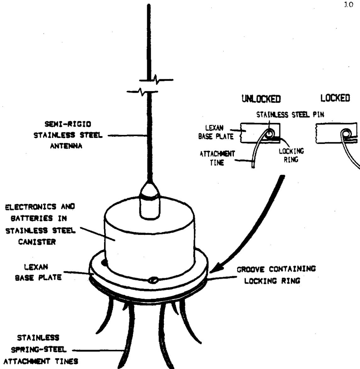
Figure 1. Diagram of the redesigned barnacle tag. Diagram is not to scale, see text for specifications and measurements.
