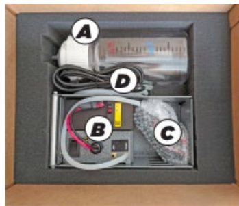
Figure 1. Citizen Scientist sampler components
