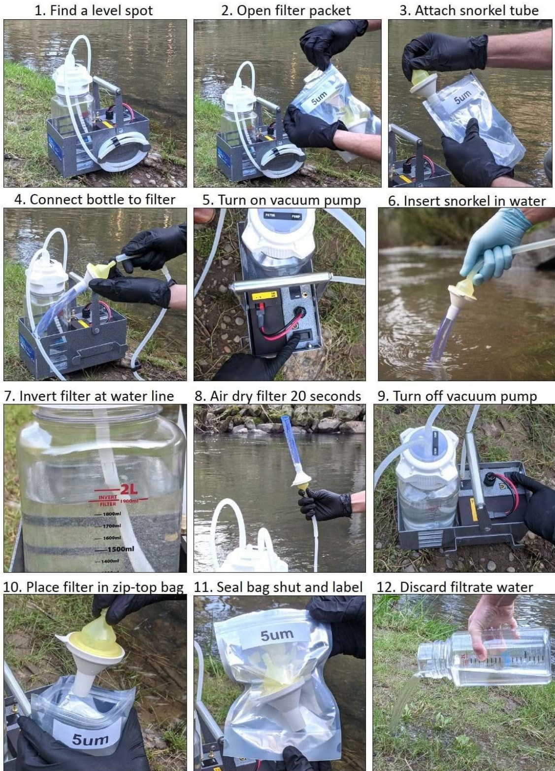
Figure 3. Visual steps for operation of the Smith-Root eDNA citizen science sampler
