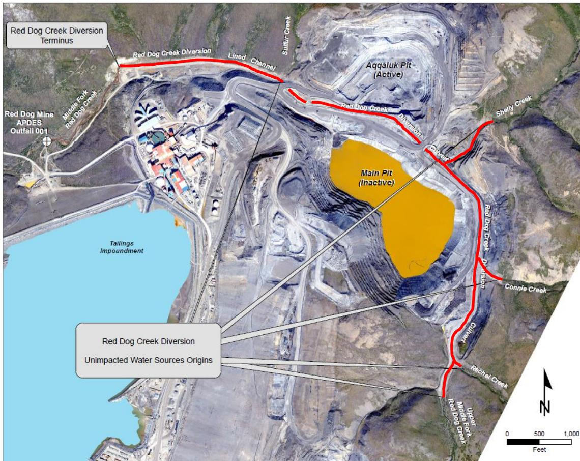
**Figure 4. Clean water bypass system at the Red Dog Mine. The Red Dog Creek diversion structure (delineated by labels in the photograph and shown in red) picks up non-mining impacted waters from upstream tributaries and moves them between the Akqaluk pit and the main pit back to the original Middle Fork Red Dog Creek streambed (flow is from right to left).<sup>2</sup>**
