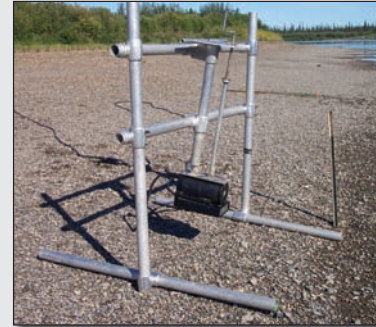
A DIDSON transducer mounted to an aluminum frame awaits deployment into the Sheenjek River.
