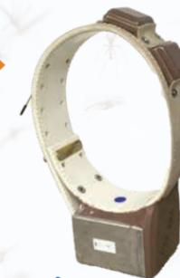
Adult caribou are fitted with **radiocollars** that record **GPS locations** determined by satellites, and transmit a **VHF radio signal** that can be picked up with a receiver and antenna nearby.
