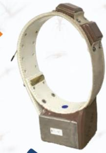
Adult caribou are fitted with **radiocollars** that record **GPS locations** determined by satellites, and transmit a **VHF radio signal** that can be picked up with a receiver and antenna nearby.
