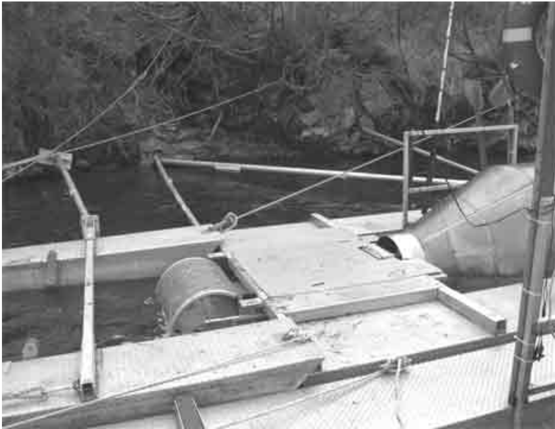
Figure 9. This photo illustrates the position of the trap legs on shore and how the pontoons of the small trap and live box work area align.
