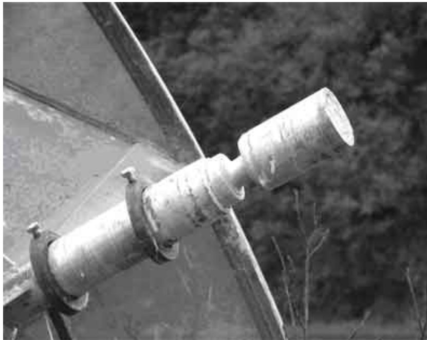
Figure 5. The photo illustrates the large trap cone spindle and O-rings. Excessive wear on the spindle can occur due to improper placement of the bipod hoist structure. Care should be taken so that the bipod hoist structure does not contact the rotating spindle. The small trap cone has a sleeve attachment.
