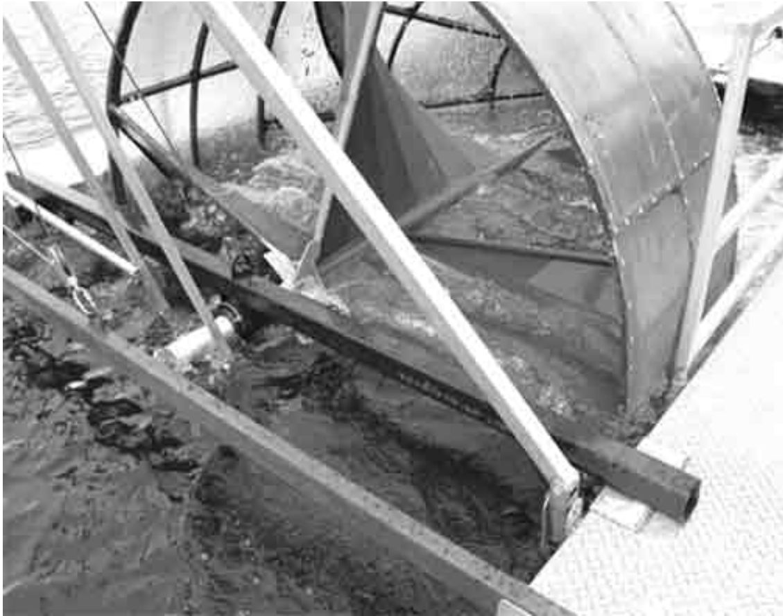
Figure 11. The assembled large trap fishing. Note that the front spindle support beam is resting on the pontoons. The spindle should be turning with little resistance inside the bushing and minimal play between the O-rings. This prevents excessive wearing of the bushing.
