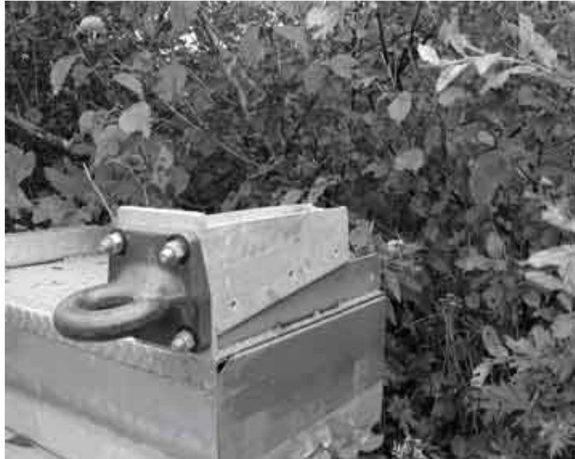
Figure 3. The photo illustrates how the pintle ring fits over a stern beam sleeve. This photo does not show the live box beams inside the sleeve.
