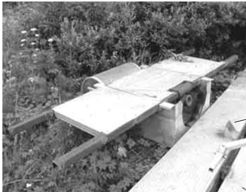
Figure 2. The photo illustrates the dual beamed live box for the large trap. The winch mount on the starboard pontoon is also visible from this angle.
