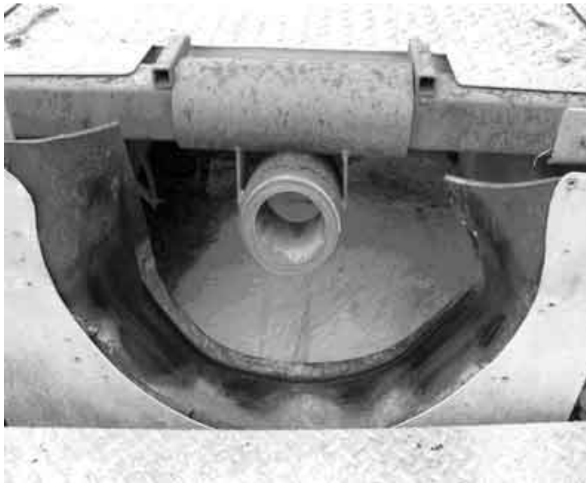
Figure 6. The picture shows the entrance to the live box and the rear spindle mount and plastic bushing. Check for excessive bushing-wear frequently throughout the season and report to project manager.
