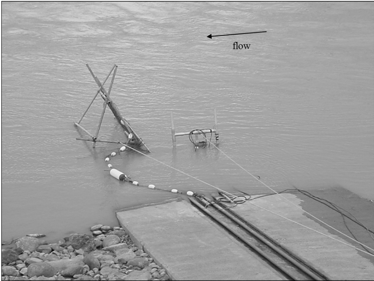
Figure 7.—The south bank weir on the downriver side of the DIDSON at the Copper River, Miles Lake sonar.
