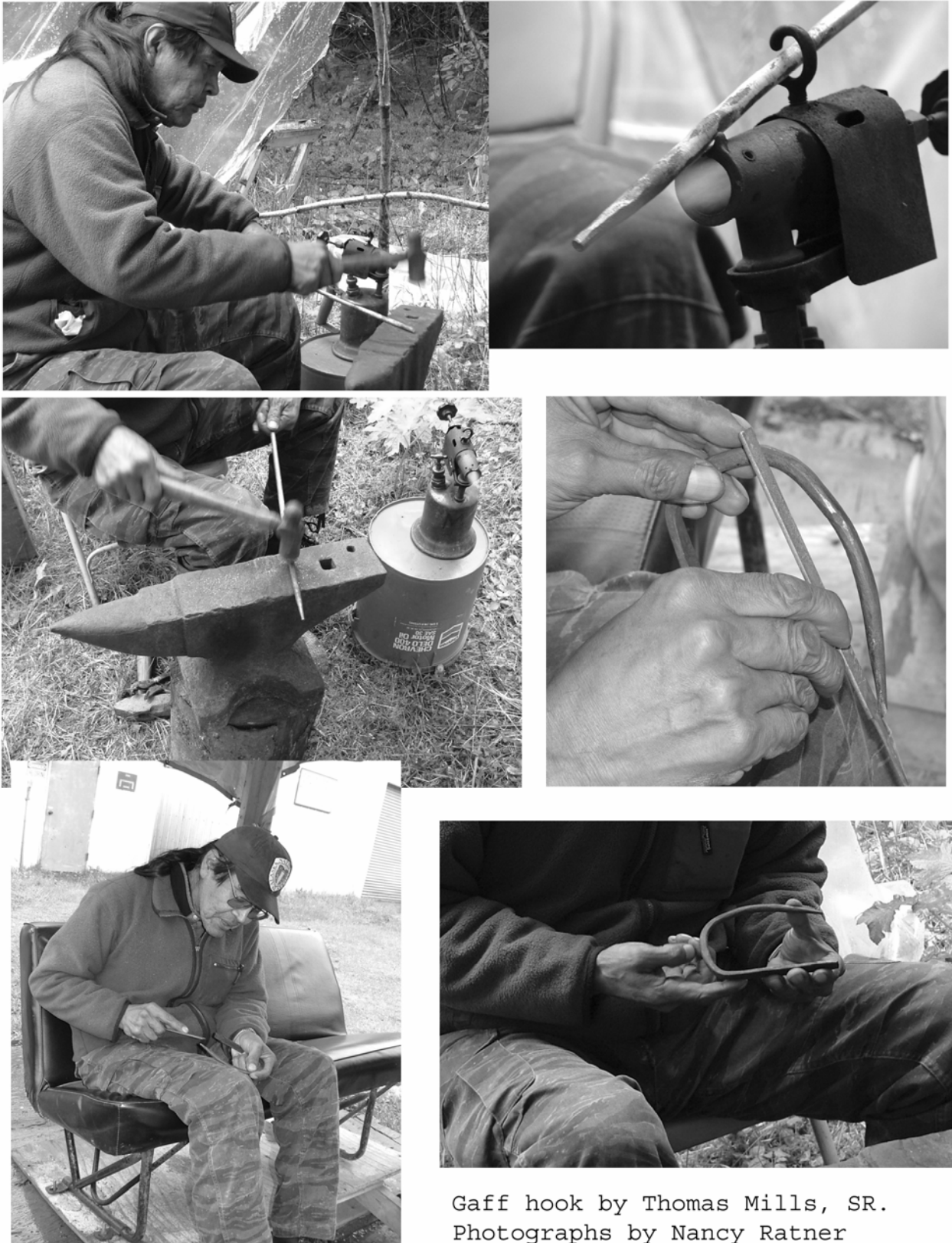
Figure E- 1. Making a Traditional Gaff Hook
