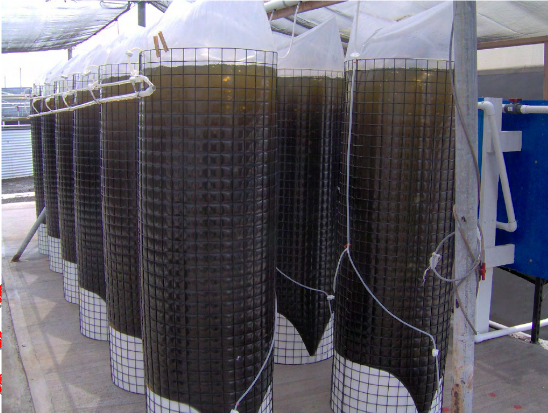
Figure 5. Bags of microalgae held up by fiberglass base and wire mesh cages.
