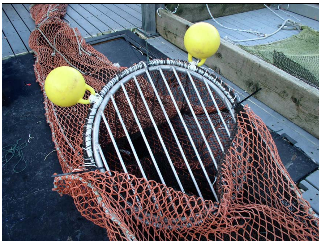
Figure 2. —Finfish-excluder device installed on the ADF&G shrimp research trawl.
