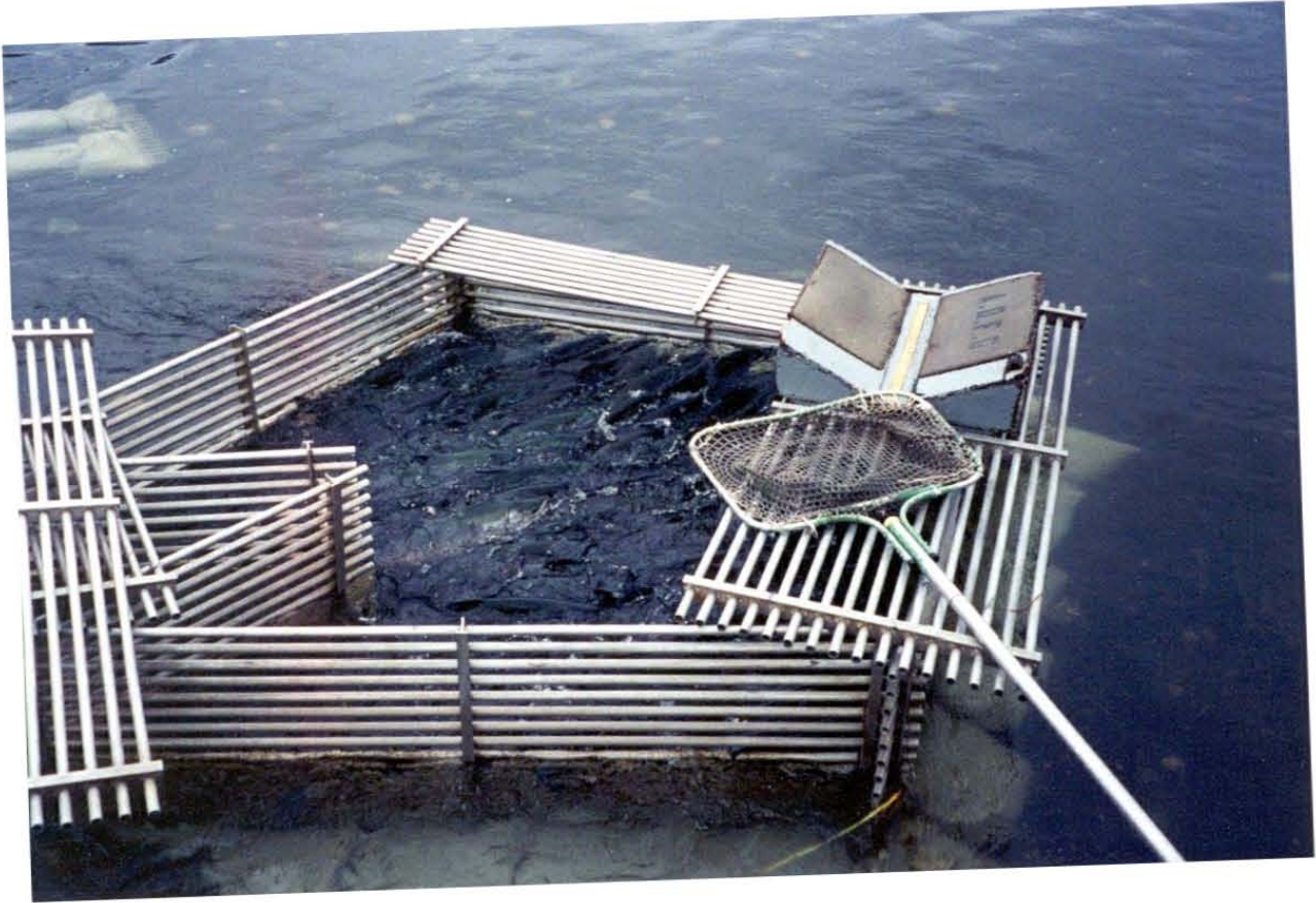
Figure 3.—Picture of weir trap setup.
