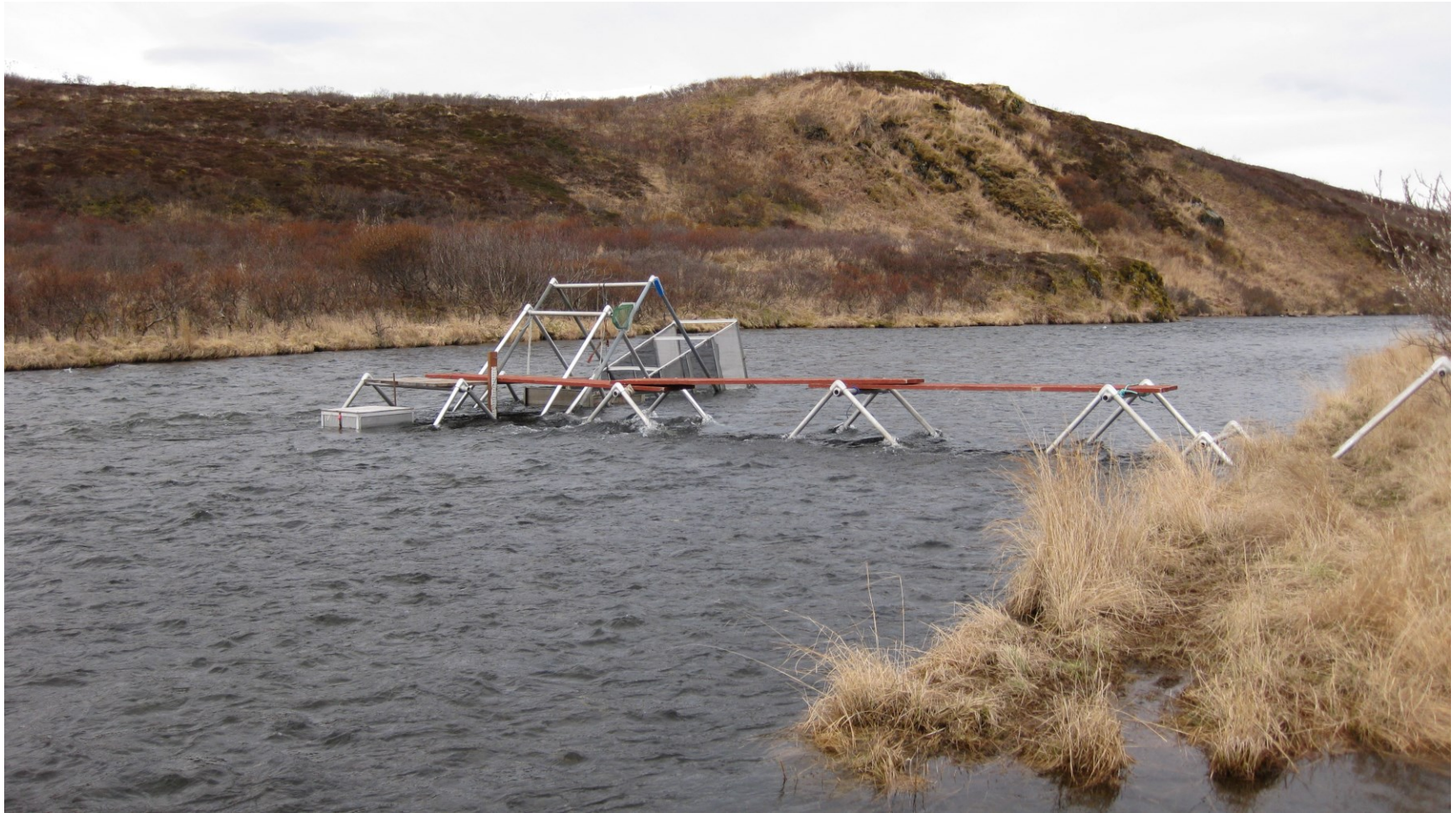
Figure 3.—Inclined plane smolt trap configuration and board walk.
