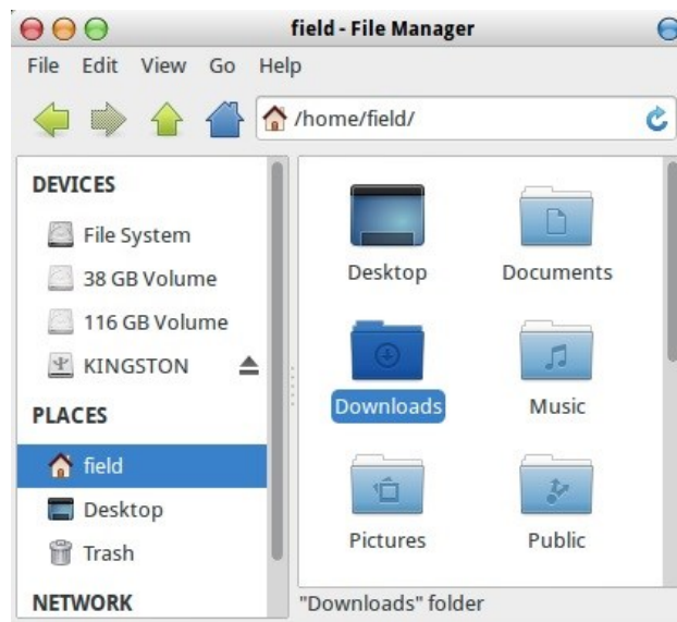
Figure 9.–The File Manager appears when you right click on the desktop and select Open in New Window. This is used for accessing the Downloads folder (under PLACES) and the USB flash drive (under DEVICES).
