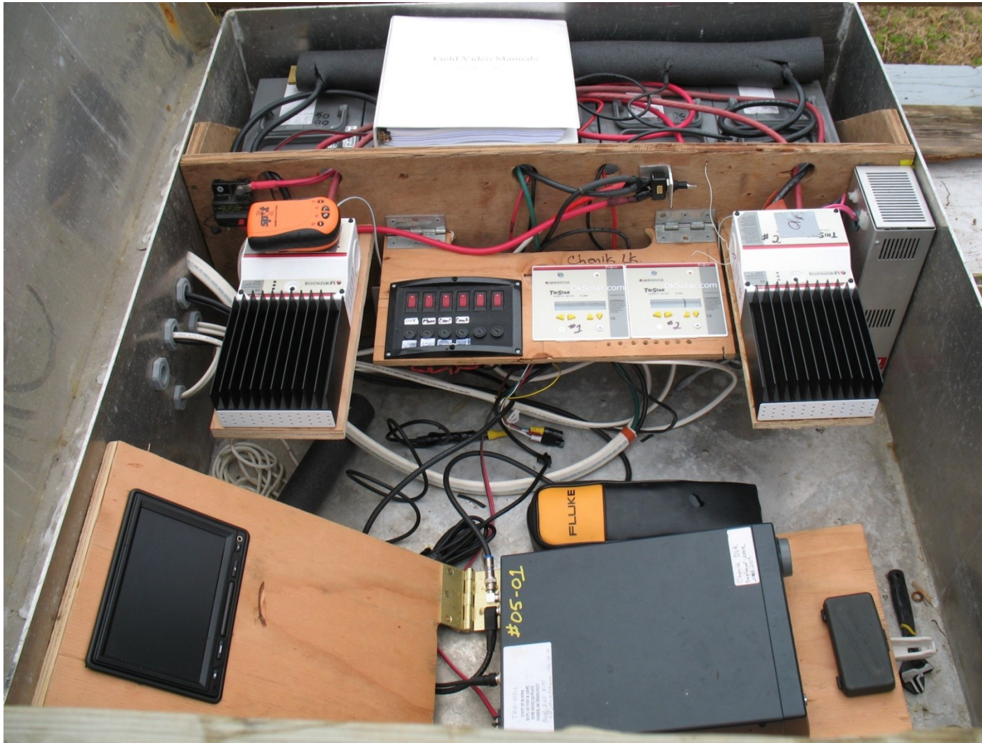
Figure 6.—Photograph illustrating the wooden "dashboard" used to isolate the batteries from sensitive electronic components and to attach and organize wiring and electronic components of the remote video system.
