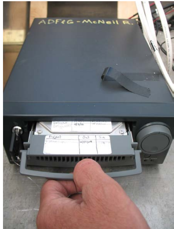
Figure 16. Photos illustrating use of key to unlock (A) and remove (B) hard drive for swapping.
