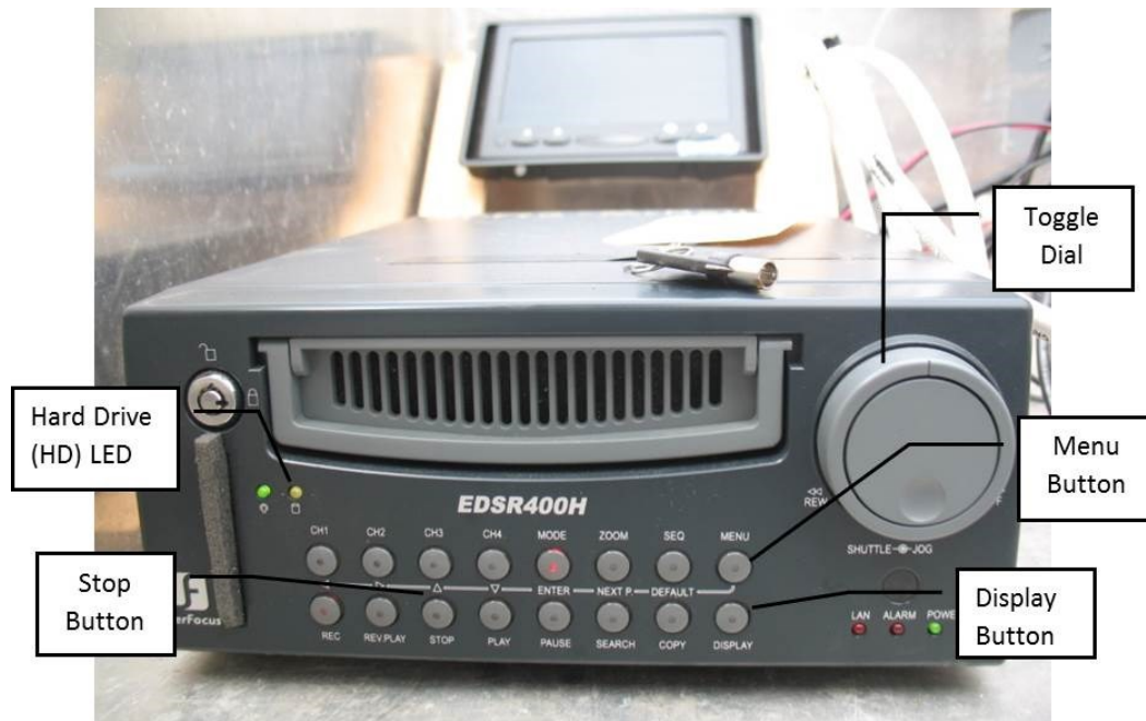
Figure 18. DVR control panel illustrating key buttons and indicator lights.
