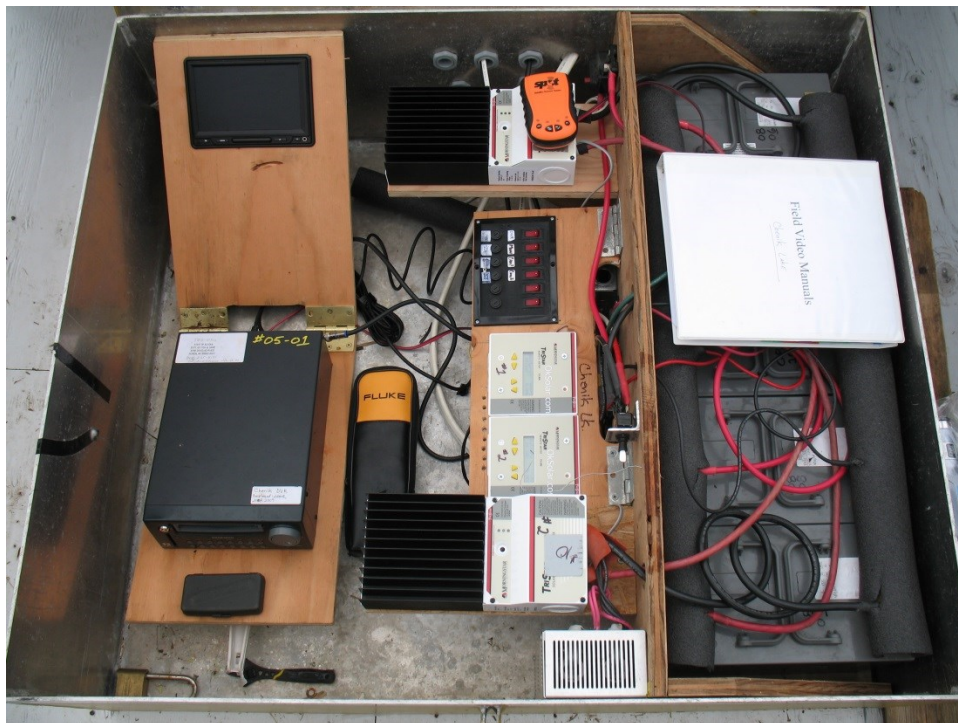
Figure 15. Layout inside strongbox allowing access to DVR controls while viewing monitor.
