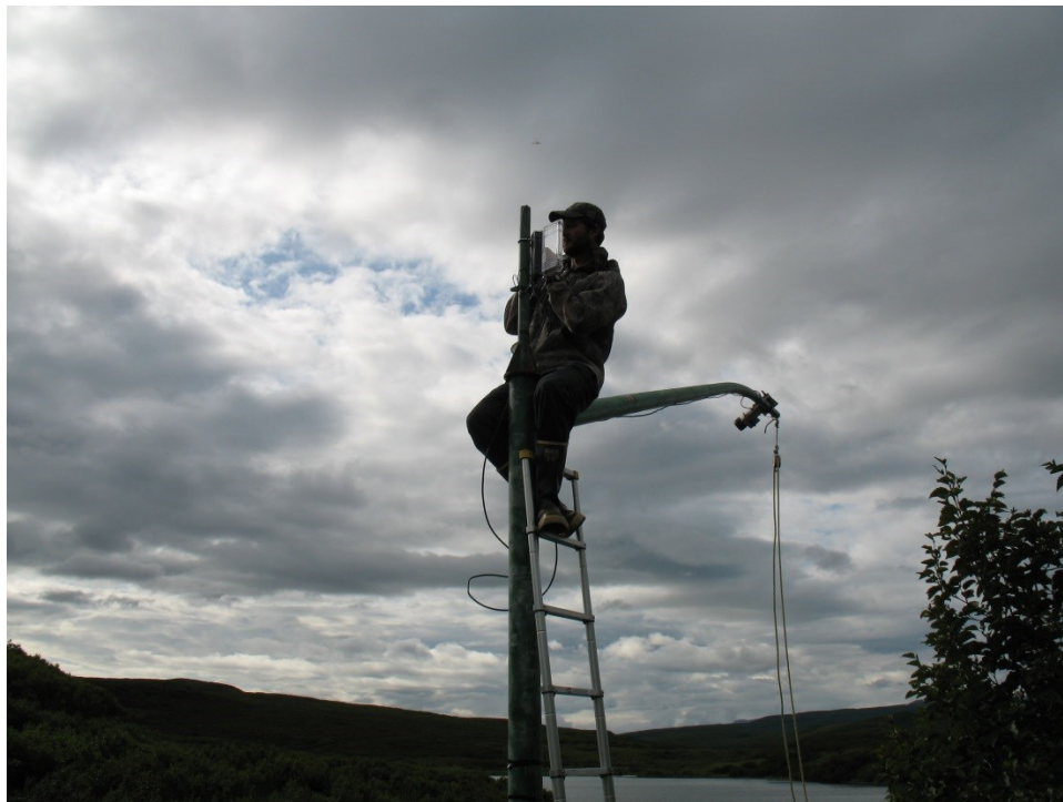
Figure 3. Accessing the Pelican case at the top of the light pole at Mikfik Creek using the collapsible ladder stored inside the creek-side strongbox.
