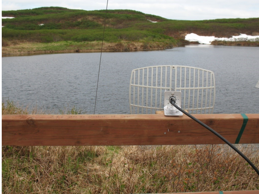
Figure 10. Microwave antenna affixed to the solar panel bracket and pointed directly at the transceiver attached to the light pole at Mikfik Creek. Note the large coax that runs into the strong box.
