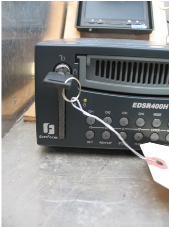
Figure 16. Photos illustrating use of key to unlock (A) and remove (B) hard drive for swapping.
