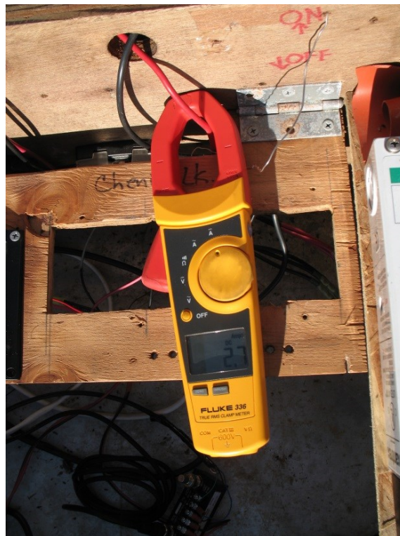
Figure 19. Use a clamp meter to check amperage gains (from solar panels and wind generator) and draws (from various electronic components) to make sure they're in the expected ranges. Note: clamp meter goes around just the positive lead.
