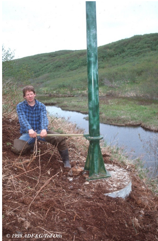
Figure 6. Use square tube pipe (stored inside box) to pivot the light pole after loosening the two bolts that secure it in place. Wrenches for loosening these bolts are stored in the box. Be sure to re-secure the pole in the new position so it won't pivot while servicing the camera.
