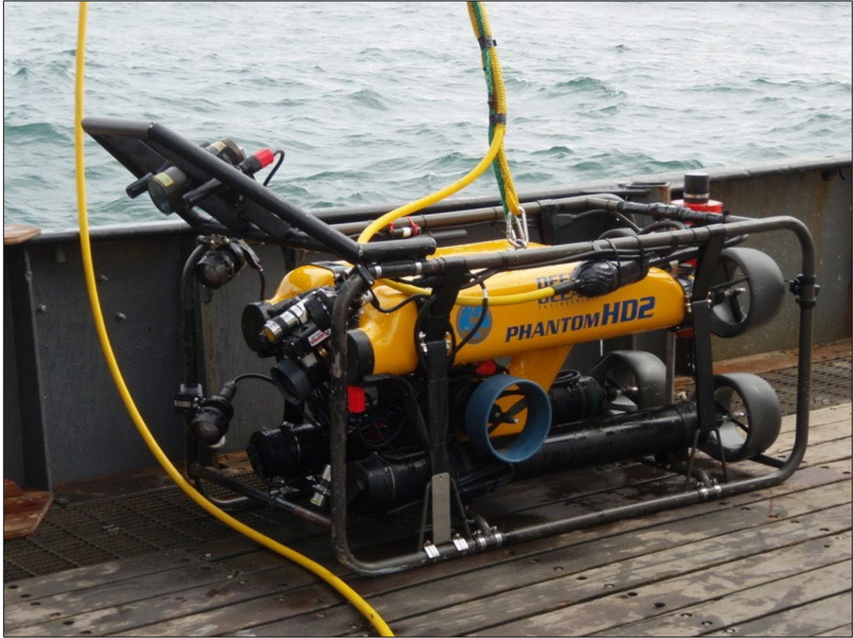
Figure 6.—Deep Ocean Engineering Phantom HD2+2 remotely operated vehicle (ROV) Buttercup used for the survey.
