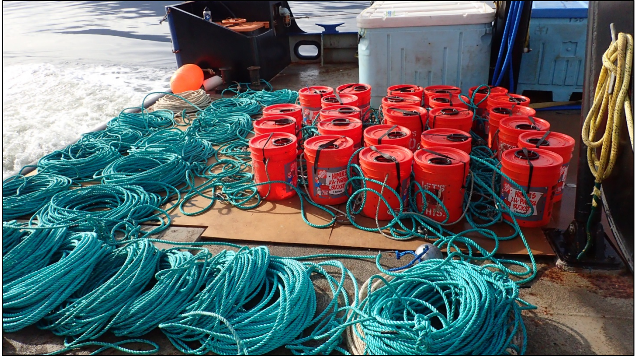
Figure 1.—Experimental longline set using 5-gallon bucket traps designed to capture Pacific and black hagfish during the Southeast Alaska pre-season shrimp survey.
