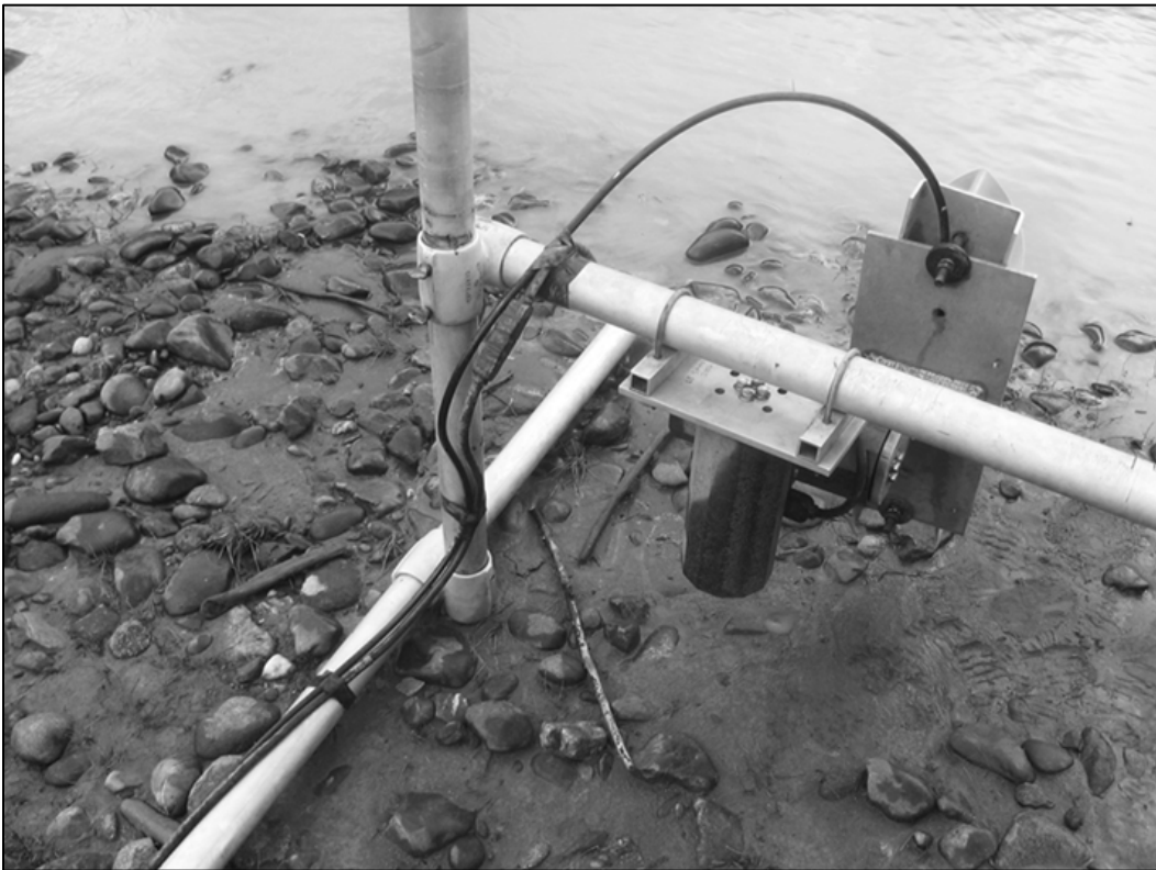
Figure 5.—Split-beam transducer mounted to an aluminum H-mount (top) and the same transducer mounted to 2 single-axis automated rotators (bottom) used on the left bank at the Eagle sonar project on the Yukon River.
