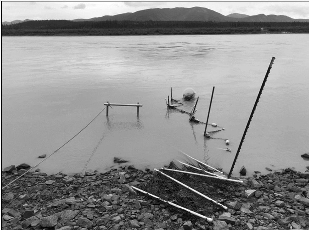
Figure 6.—Portable tripod-style fish lead used on the left bank (top) and seine mesh fish lead used on the right bank (bottom) at the Eagle sonar project on the Yukon River.
