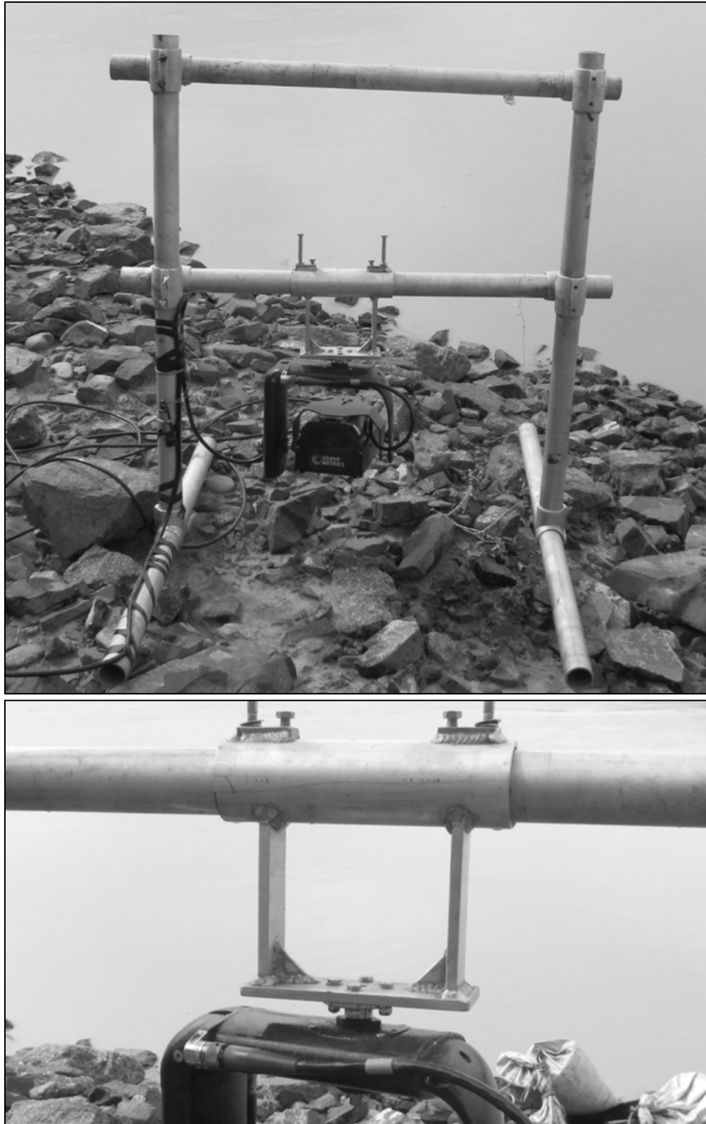
Figure 7.—Adaptive resolution imaging sonar (ARIS) and AR2 Rotator mounted to an aluminum H-mount (top) and close-up view of rotator mount (bottom) at the Eagle sonar project on the Yukon River.
