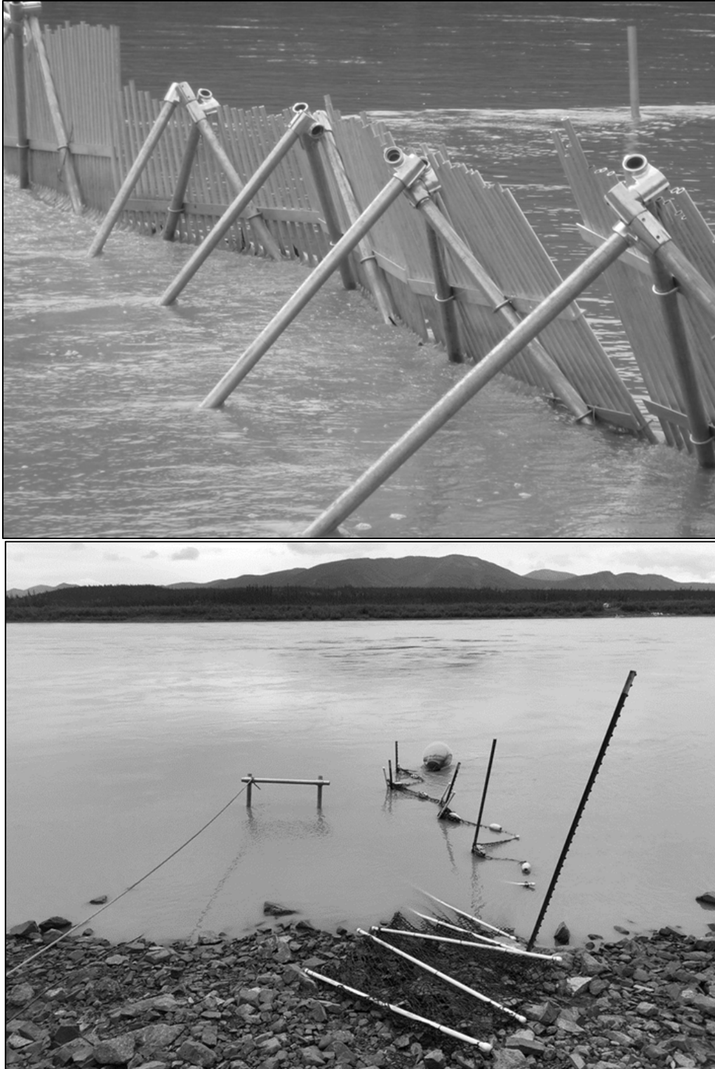
Figure 6.—Portable tripod-style fish lead used on the left bank (top) and seine mesh fish lead used on the right bank (bottom) at the Eagle sonar project on the Yukon River.
