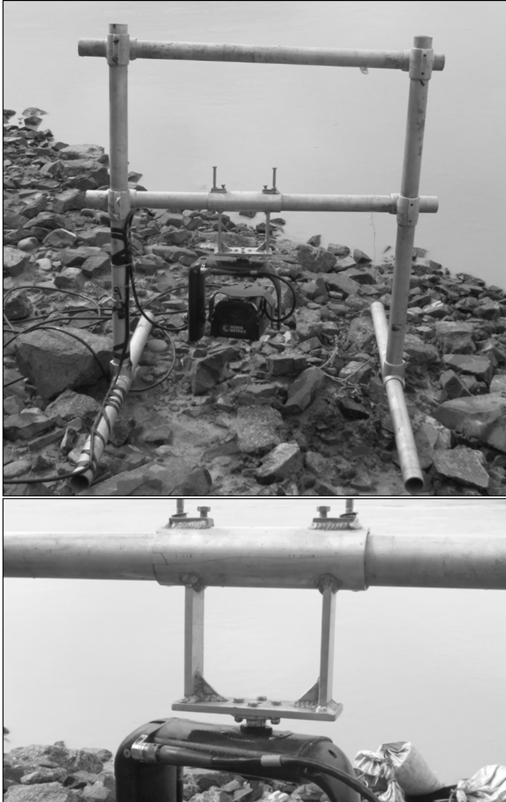
Figure 7.—ARIS imaging sonar and AR2 Rotator mounted to an aluminum H-mount (top) and close-up view of rotator mount (bottom) at the Eagle sonar project on the Yukon River.
