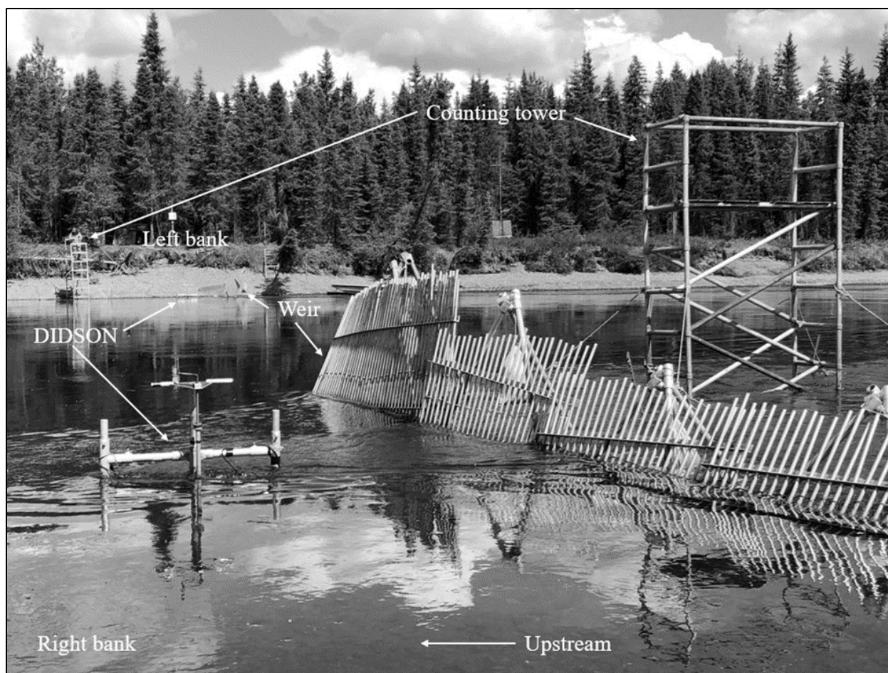
Figure 5.—Anvik River sonar project site illustrating locations of sonars, weirs, and counting towers.
