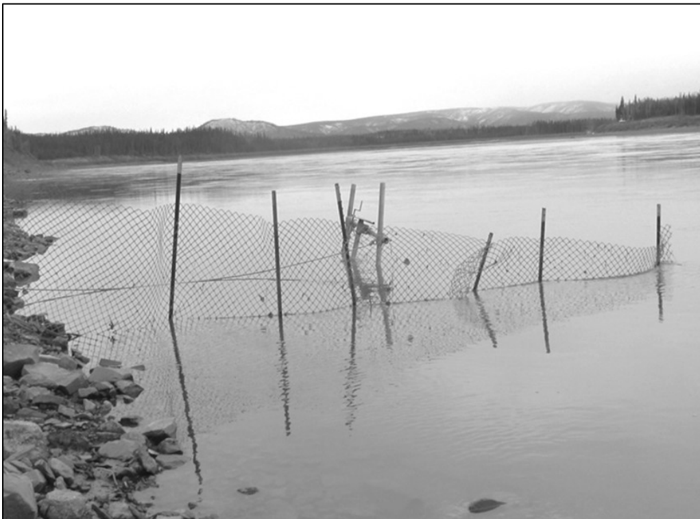
Figure 6.—Portable tripod-style fish lead used on the left bank (top) and snow fence fish lead used on the right bank (bottom) at the Eagle sonar project on the Yukon River.
