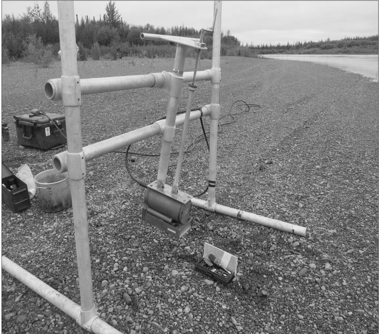
Figure 4.—View of a DIDSON (dual-frequency identification sonar) mounted to an aluminum pod with a manual crank-style rotator at the Sheenjek River sonar project.
