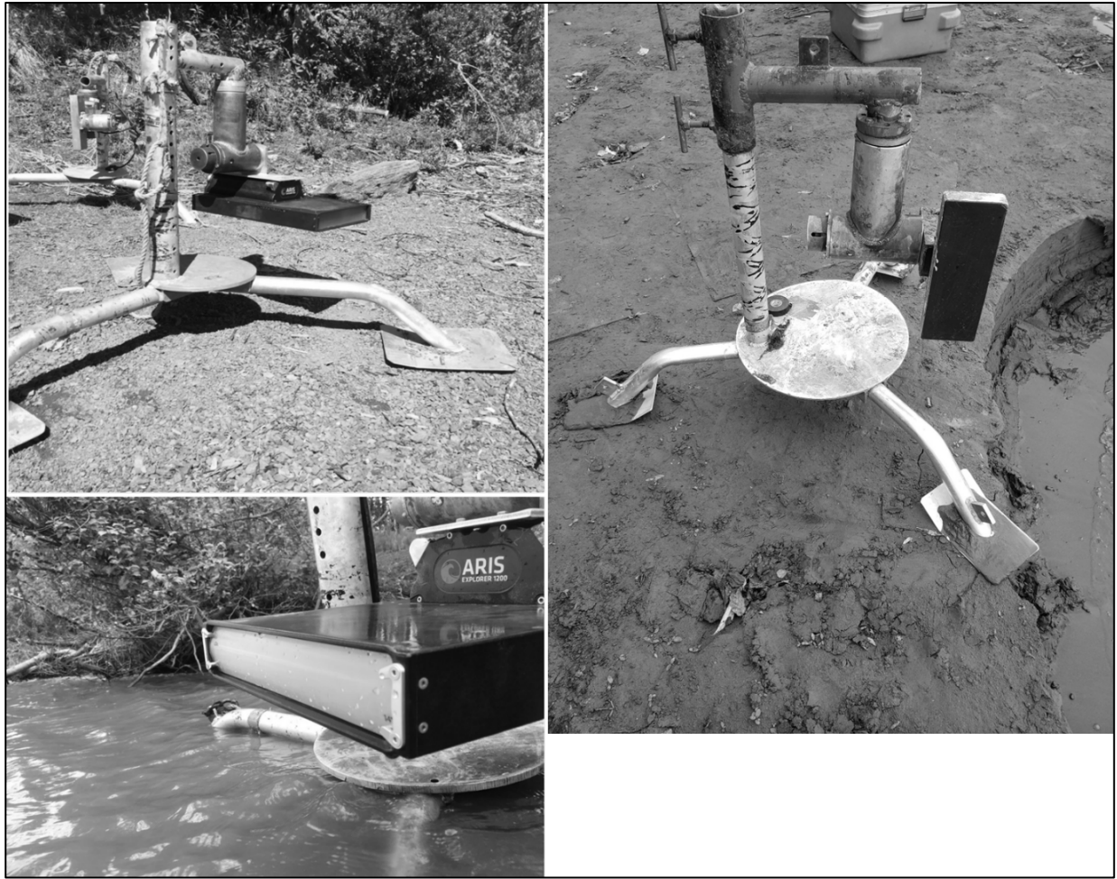
Figure 8.—ARIS with a telephoto lens mounted to a pod with PT-25 rotator (top left), ARIS with spreader lens installed on the front of the telephoto lens (lower left), and HTI split beam transducer mounted on the pod with PT-25 rotator (right), at the Pilot Station sonar project on the Yukon River.
