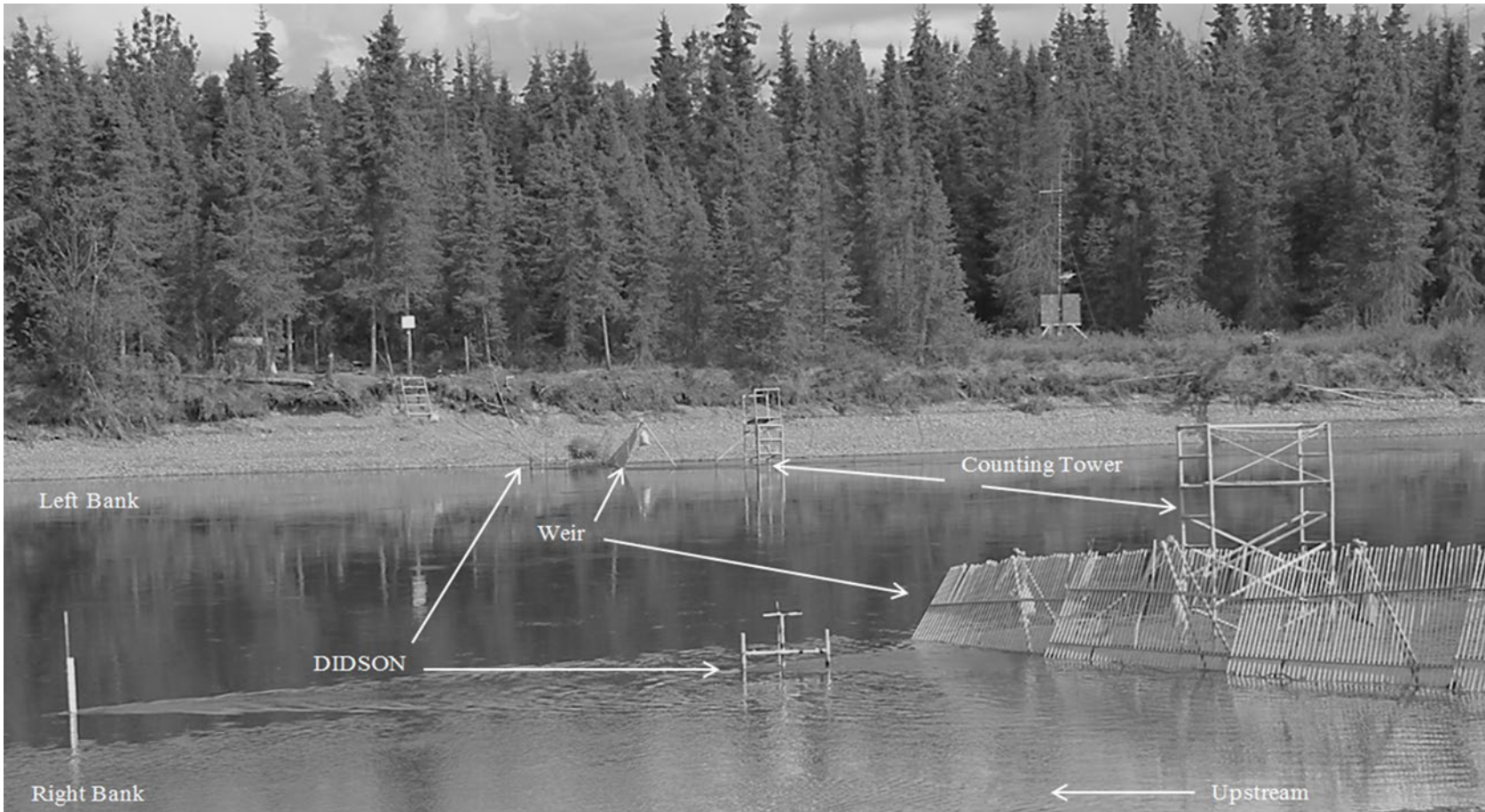
Figure 6.—Anvik River sonar project site illustrating locations of sonars, weirs, and counting towers.
