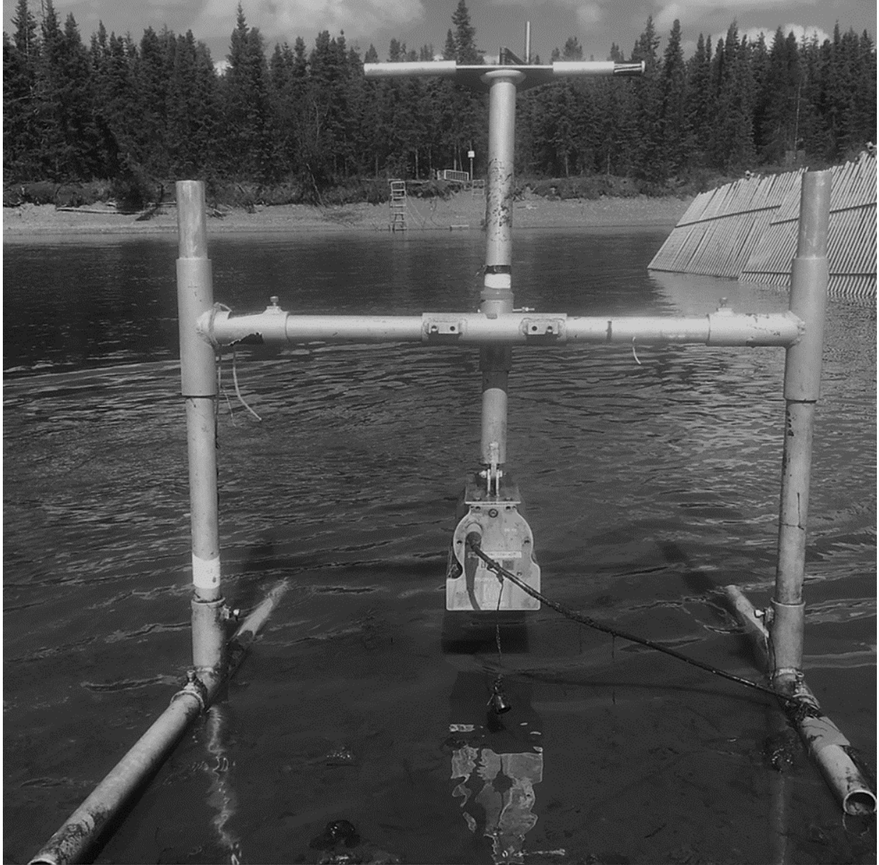
Figure 5.–View of a dual-frequency identification sonar (DIDSON) mounted to aluminum H-mount with manual crank-style rotator at the Anvik River sonar project.
