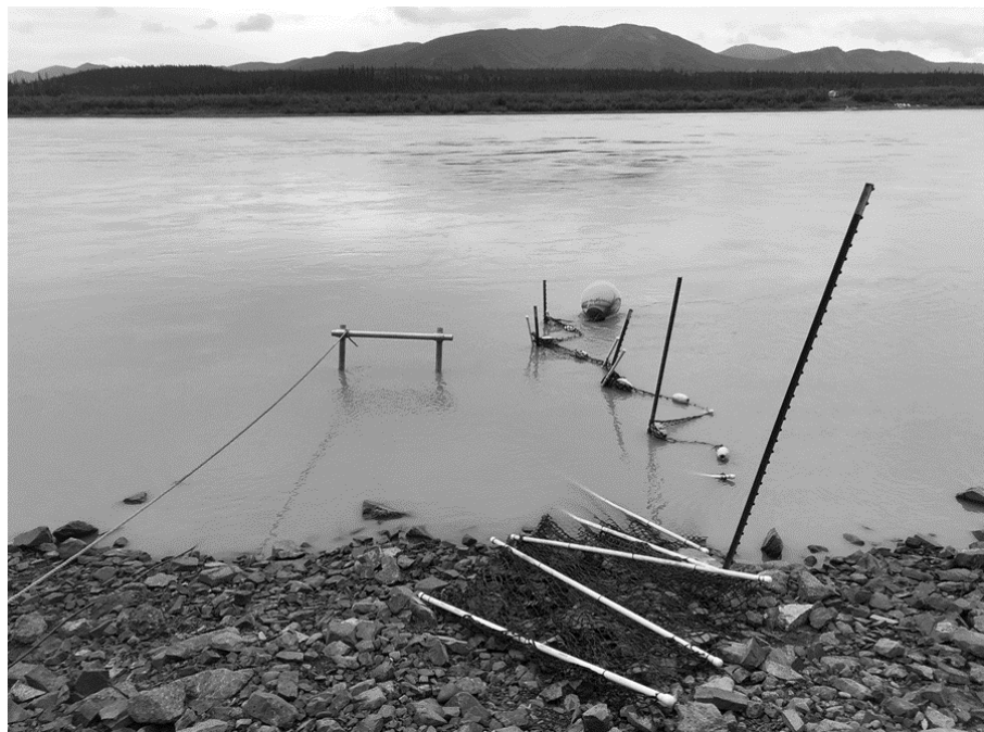
Figure 6.—Portable tripod-style fish lead used on the left bank (top) and seine mesh fish lead used on the right bank (bottom) at the Eagle sonar project on the Yukon River, 2020.
