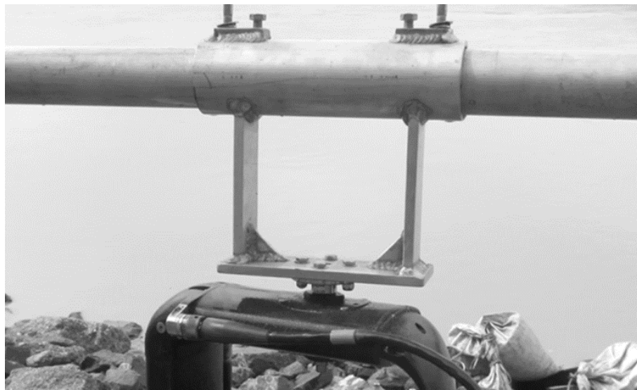
Figure 7.—ARIS imaging sonar and ARIS Rotator AR2 mounted to an aluminum H-mount (top) and close-up view of rotator mount (bottom) at the Eagle sonar project on the Yukon River, 2020.
