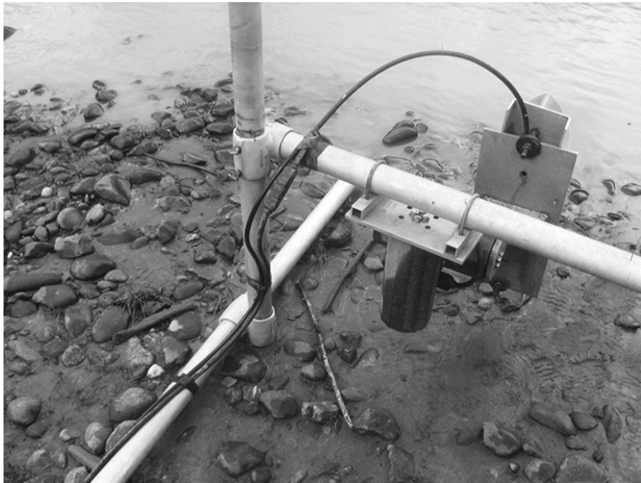
Figure 5.—Split-beam transducer mounted to an aluminum H-mount (top) and the same transducer mounted to 2 single-axis automated rotators (bottom) used on the left bank at the Eagle sonar project on the Yukon River, 2020.
