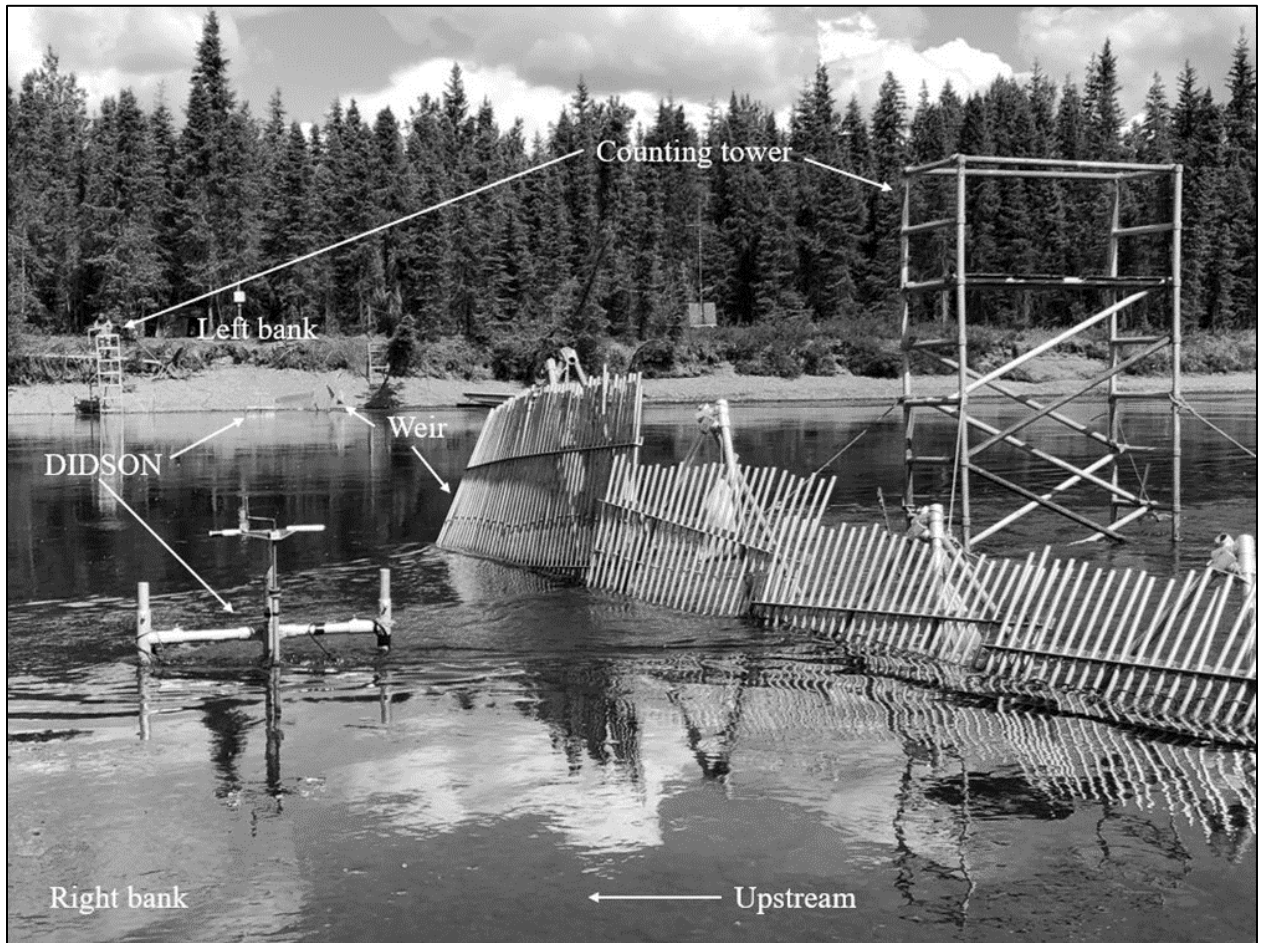
Figure 5.—Anvik River sonar project site illustrating locations of sonars, weirs, and counting towers, 2022.
