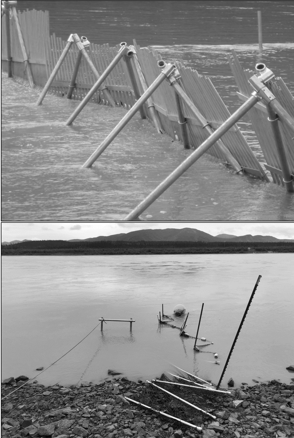
Figure 6.—Portable tripod-style fish lead used on the left bank (top) and seine mesh fish lead used on the right bank (bottom) at the Eagle sonar project on the Yukon River, 2022.
