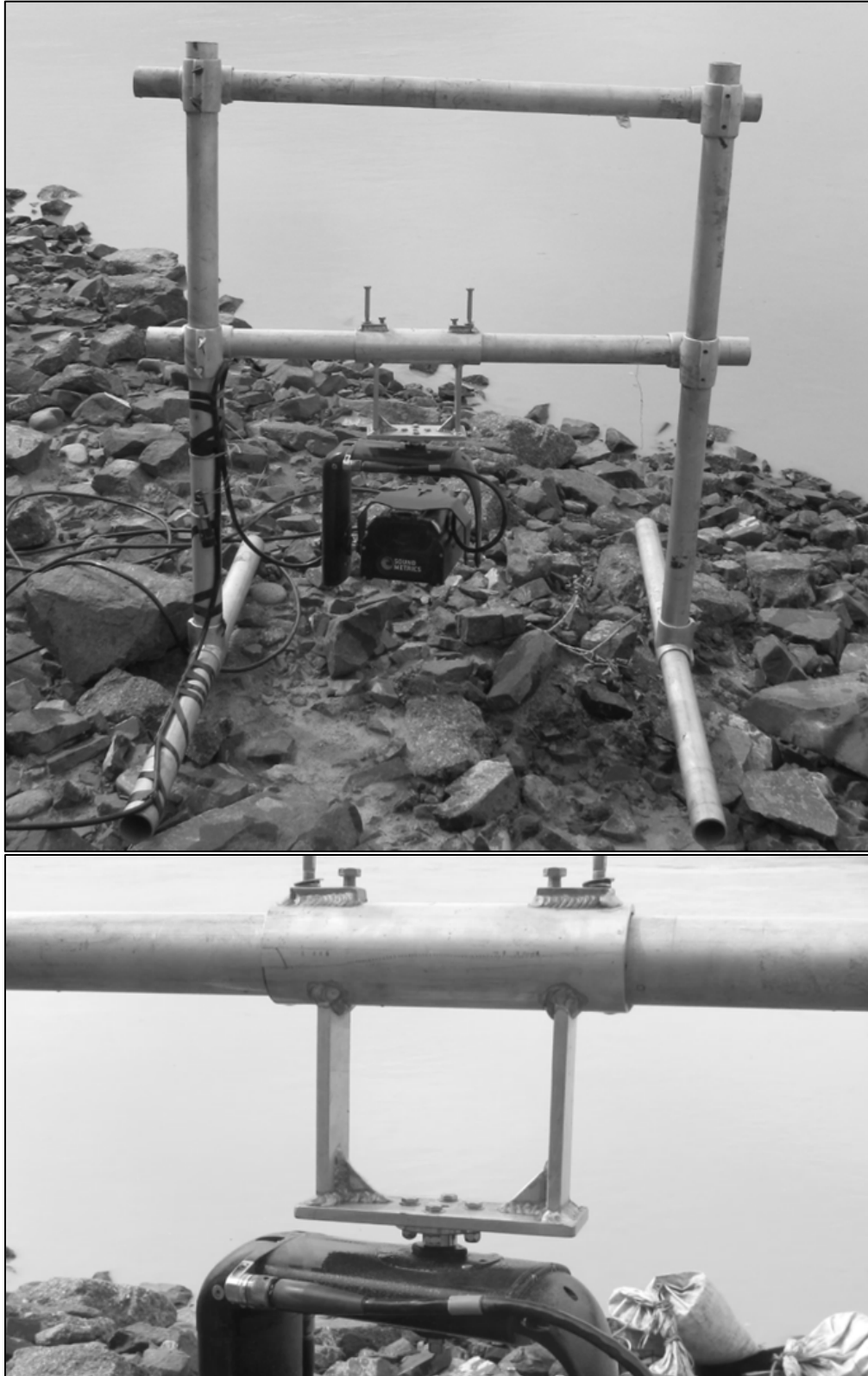
Figure 7.—ARIS imaging sonar and AR2 Rotator mounted to an aluminum H-mount (top) and close-up view of rotator mount (bottom) at the Eagle sonar project on the Yukon River, 2022.
