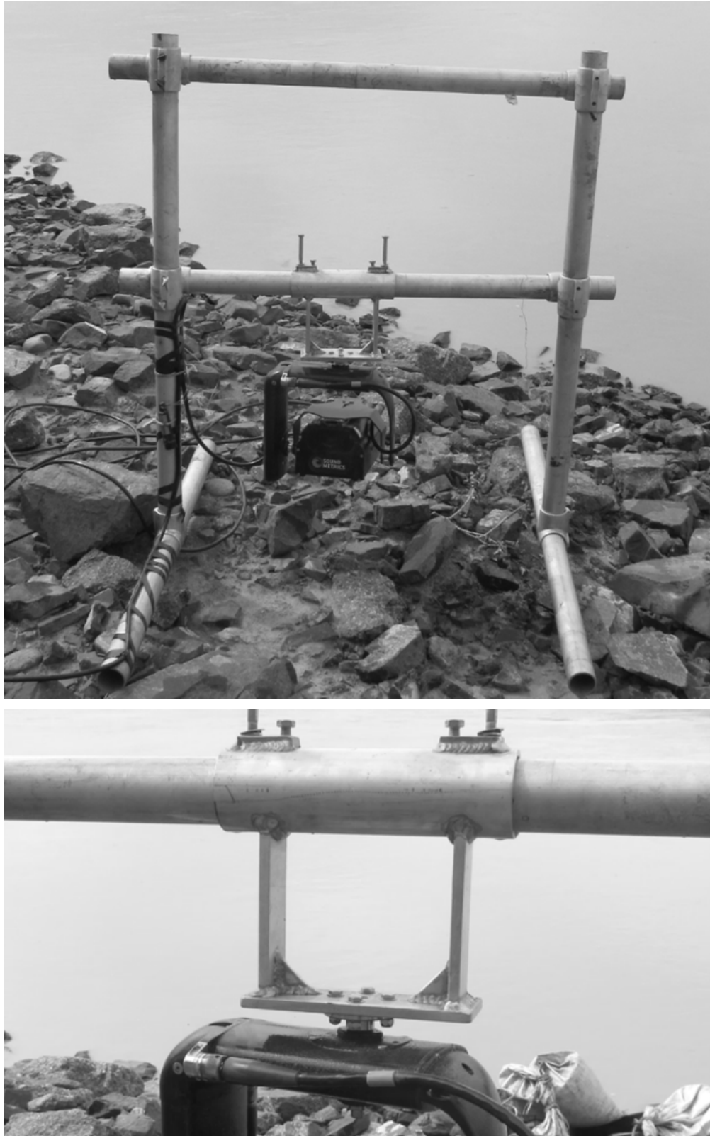
Figure 7.—ARIS imaging sonar and ARIS Rotator AR2 mounted to an aluminum H-mount (top) and close-up view of rotator mount (bottom) at the Eagle sonar project on the Yukon River, 2019.
