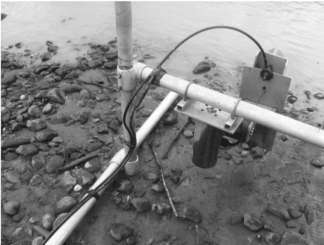
Figure 5.—Split-beam transducer mounted to an aluminum H-mount (top) and the same transducer mounted to 2 single-axis automated rotators (bottom) used on the left bank at the Eagle sonar project on the Yukon River, 2019.
