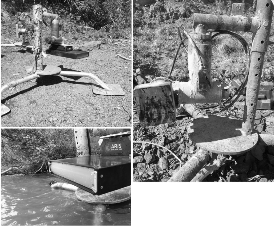
Figure 8.—ARIS with telephoto lens mounted to pod with PT-25 rotator (top left), ARIS with spreader lens installed on the front of the telephoto lens (lower left), and HTI split beam transducer mounted on pod with PT-25 rotator (right), at the Pilot Station sonar project on the Yukon River.
