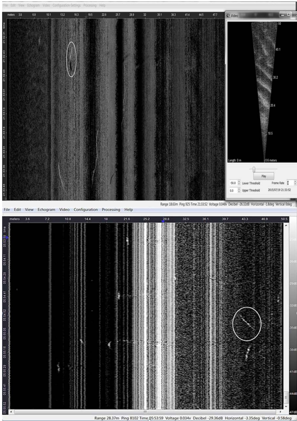
Figure 9.—Echogram of ARIS alongside video image (top) and split-beam sonar (bottom), with oval around representative fish.
