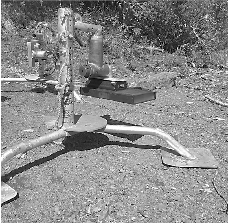
Figure 8.—Split-beam transducer mounted to pod with 662H dual axis rotators (top), and ARIS with telephoto lens mounted to pod with PT-25 rotator (bottom), at the Pilot Station sonar project on the Yukon River.
