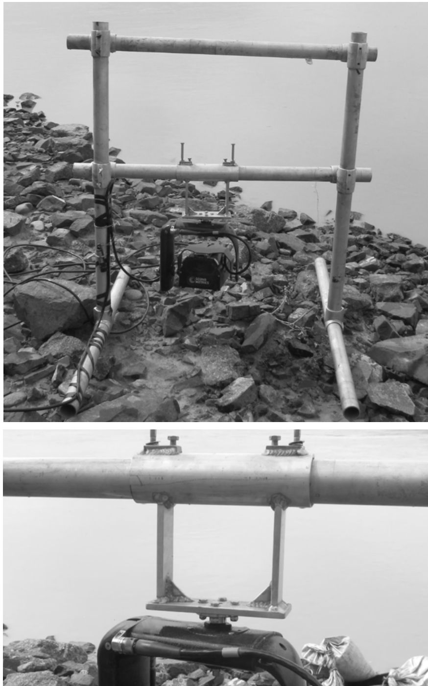
Figure 7.—View of ARIS imaging sonar and AR2 rotator mounted to an aluminum H mount (top), and closeup view of mount for rotator (bottom), at the Eagle sonar project on the Yukon River, 2017.
