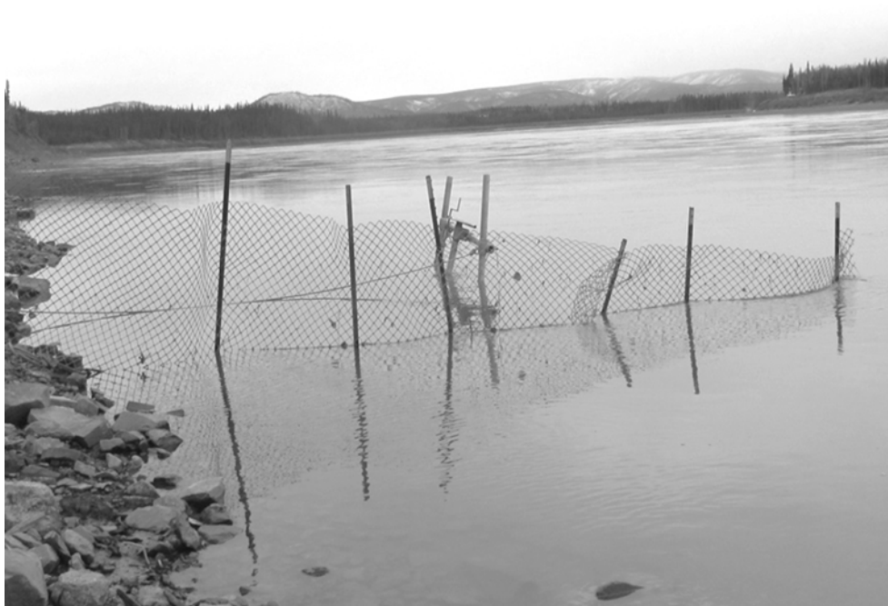
Figure 6.—Portable tripod-style fish lead used on the left bank (top) and plastic snow fencing used on the right bank at the Eagle sonar project, on the Yukon River, 2017.
