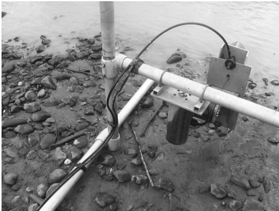
Figure 4.–Split-beam transducer mounted to an aluminum H-mount (top) and the same transducer mounted to 2 single-axis automated rotators (bottom), used on the left bank at the Eagle sonar project, on the Yukon River, 2017.
