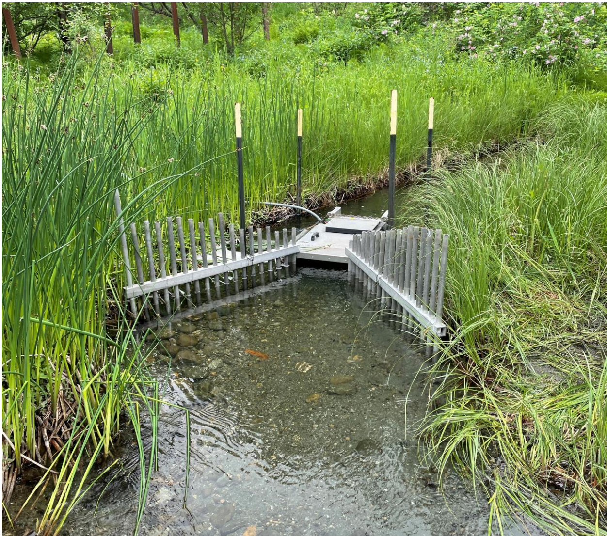
Figure 2. Vaki Riverwatcher Installation. AERC, 2022
