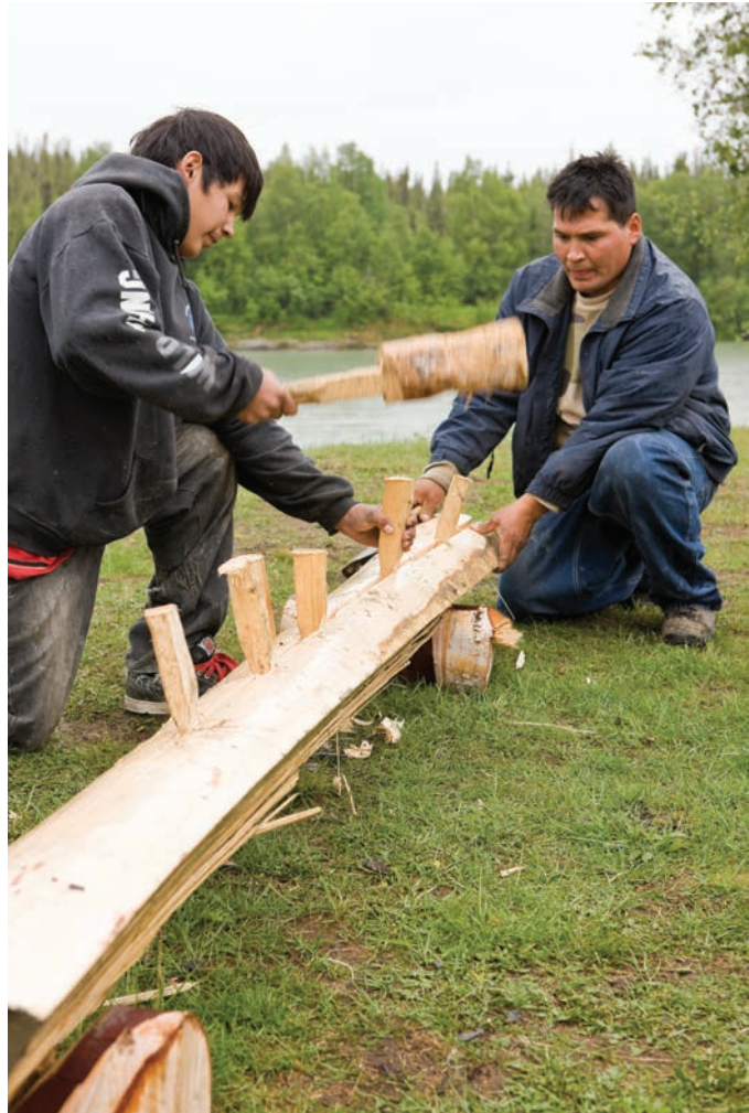
Plate 3-26.—Wayne Dick and Bryan Willis on a bank of the Stony River driving wooden wedges into a section of spruce log to make the slats for a tiz'in. Photo by Chris Arend/Anchorage Museum.
