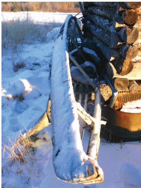
Plate 3-12.—A spruce framed canoe made by Lime Village residents. This canoe is stored behind a storage cache in Lime Village but is no longer in use. Remains of canvas that once covered the frame can be seen on left side of the canoe. Photo by James M. Van Lanen, ADF&G.
