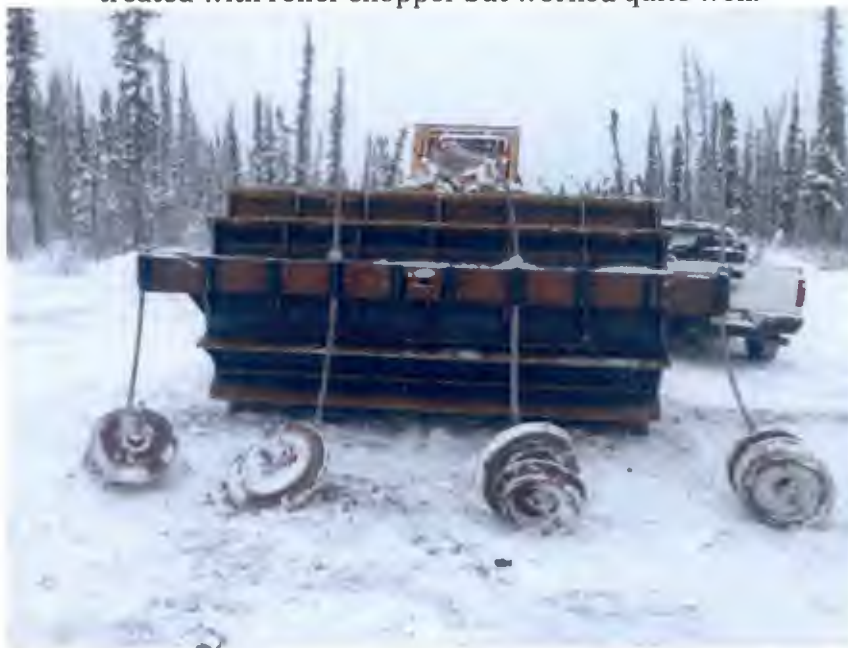
Figure B2. Modification to roller chopper in attempt to get greater scarification of moss and duff layers while roller chopping.
