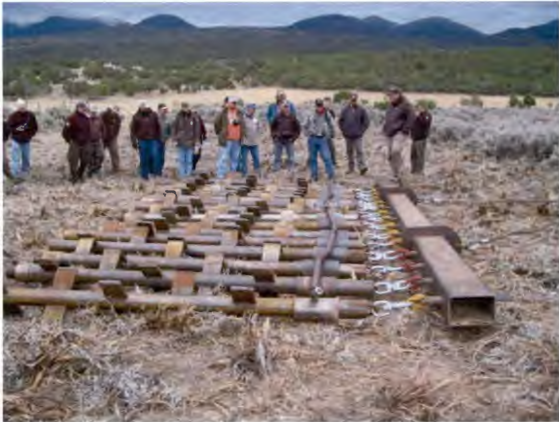
Figure B11. Dixie Pipe Harrow in western US: Design would be modified significantly for pulling behind a Roller Chopper, but concept is the same. The goal is for the pipes to spin and while cutting through the moss. Fewer pipes would be used to prevent clogging with chopped materials.
