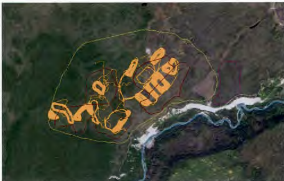
Figure A5. Klutina GPS output on areas roller chopped fall 2014 in gold, area boundary in yellow and contract treatment units in red. Note how the contractor was able to select in and around the contracted areas.
