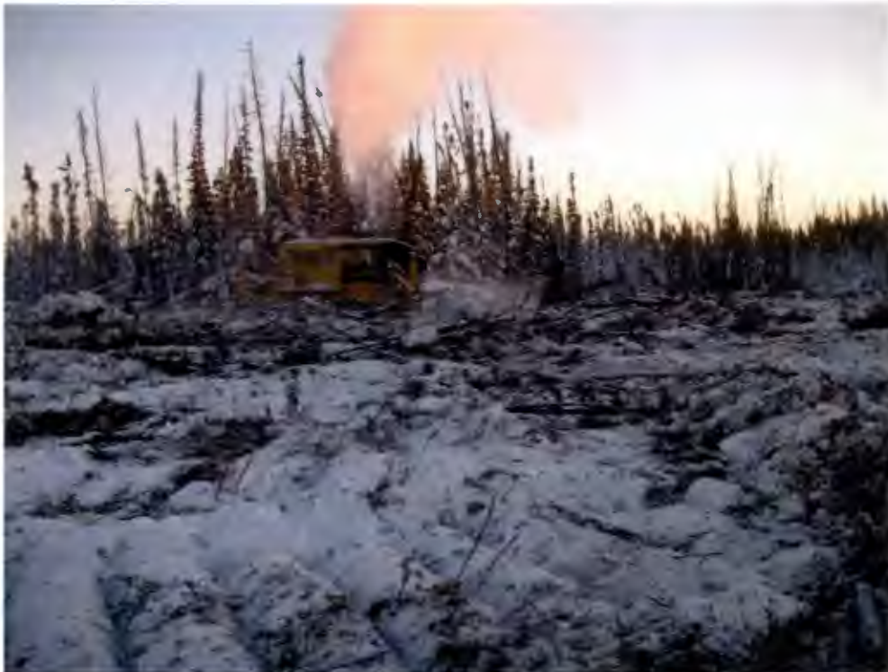
Figure B8. D-9 shearing into windrows where the stand is too large and thick to use roller chopper
