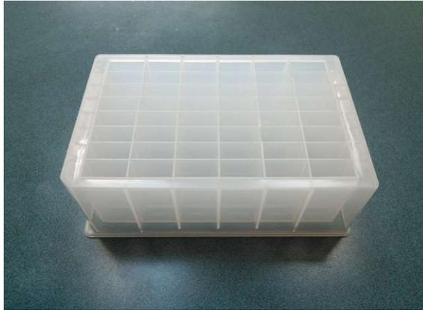
**Figure B1.** An empty 48dwp tray for DNA tissue and otoliths (cover off).
