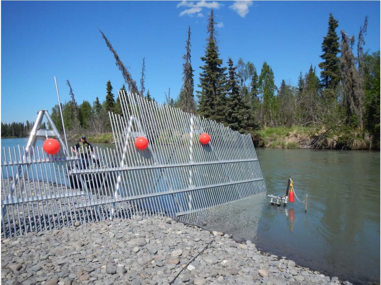
Figure 7.—Sonar coverage of the minor channel at the RM 13.7 sonar site was achieved using an ARIS 1200 deployed on a tripod mount combined with a fixed weir.
