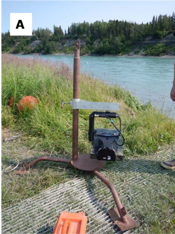
Figure 8.—An ARIS 1200 with a high-resolution lens mounted on a steel tripod for offshore deployment (A) and on an aluminum H-mount for nearshore deployment (B).
