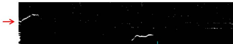
Fish is actively migrating through the beam as the sample starts. It crosses the center line and exits upstream so should be measured.
