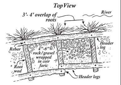
6 Install dormant cuttings 15 stems per linear foot over wrapped soil. Deposit layer of top soil over cuttings. Water liberally and
