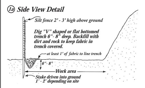
Moniter integrity of installed silt fence and remove sediment before it reaches 1/3 the height of the silt fence. It is especially important to moniter during and after rain and break-up events.
