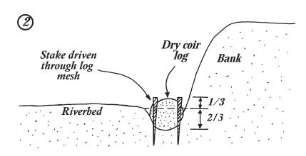
Install coir log during periods of dry riverbed or isolate area (See silt fence installation). Secure log with wooden or live stakes woven through coir log mesh and driven into earth. Stake log into place every foot on both sides. Tie adjacent logs together with biodegradable twine. Compact soil around logs. Secure the upstream and downstream ends by positioning coir logs so they transition smoothly into a stabilized bank.
