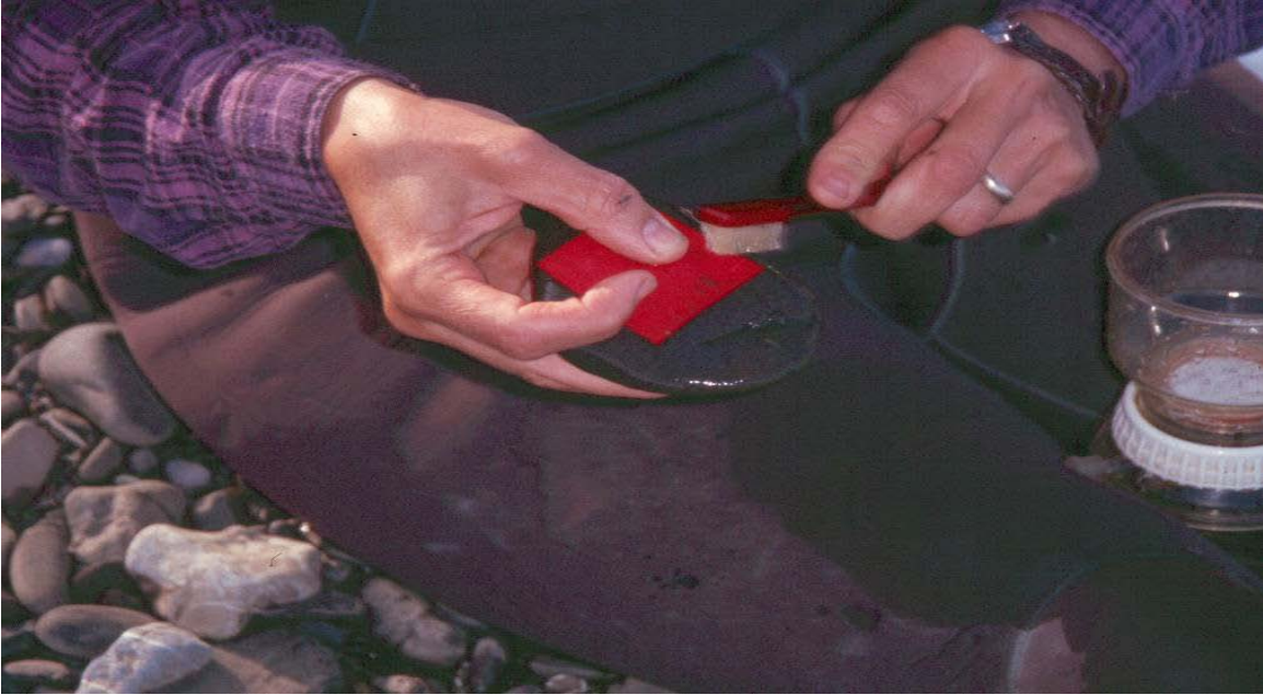
Figure 3. Brushing/removal of material from rock around the 5-cm x 5-cm flexible foam square.
