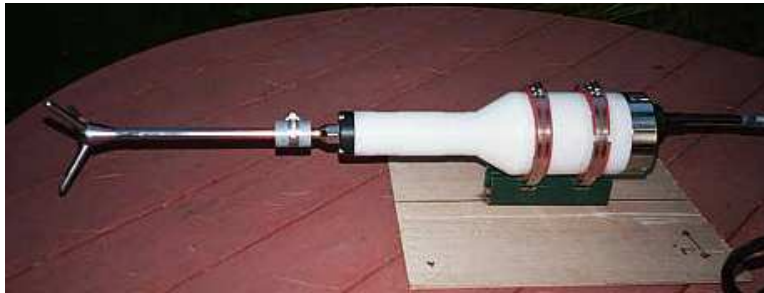
Figure 4.23: Sontek acoustic doppler velocimeter, in ‘side-looking’ mode.
