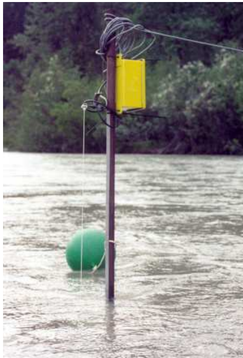
Figure 4.25: WG-50 capacitance wave gage, manufactured by Richard Brancker, Ltd.
