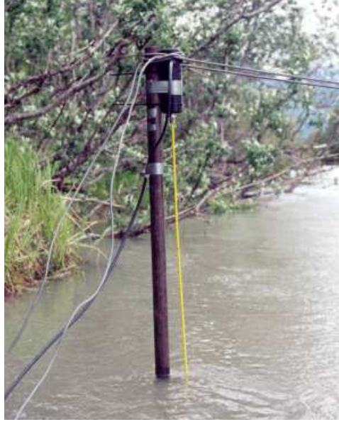
Figure 4.26: OSS capacitance wave gage, manufactured by Ocean Sensor Systems.
