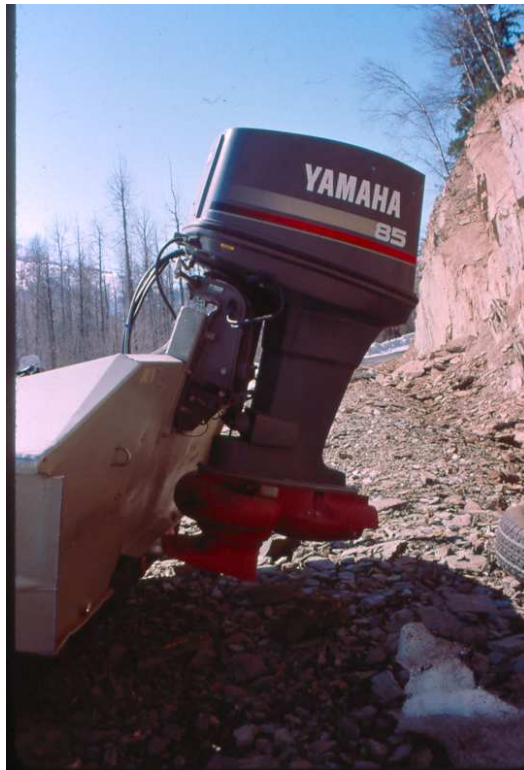
Figure 4.15: Jet-drive outboard motor.
