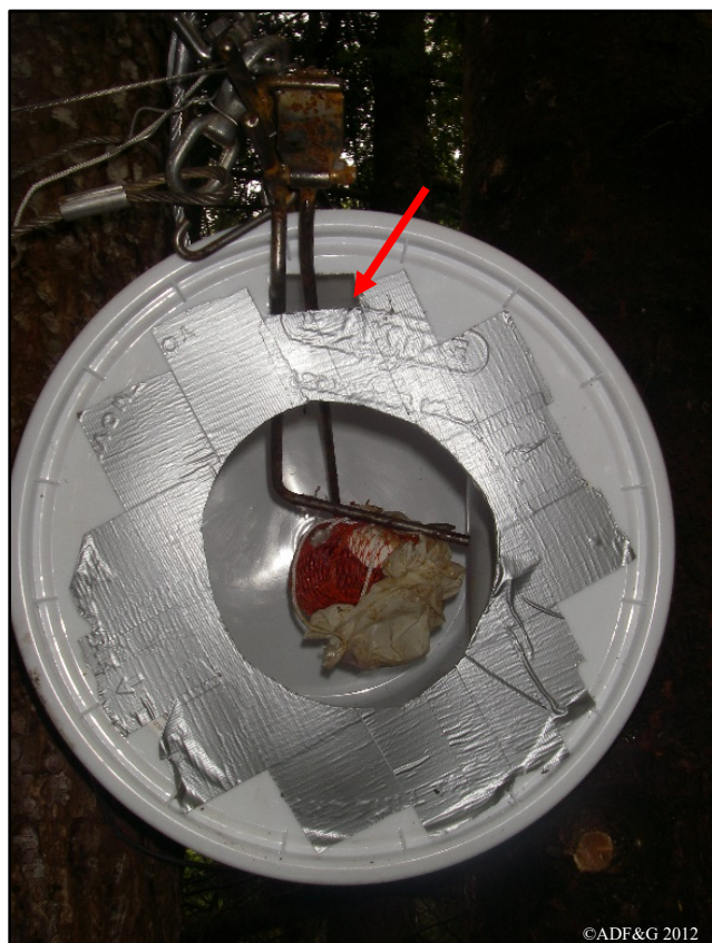
Figure 4. Hole for trigger assembly and duct tape reinforcement
