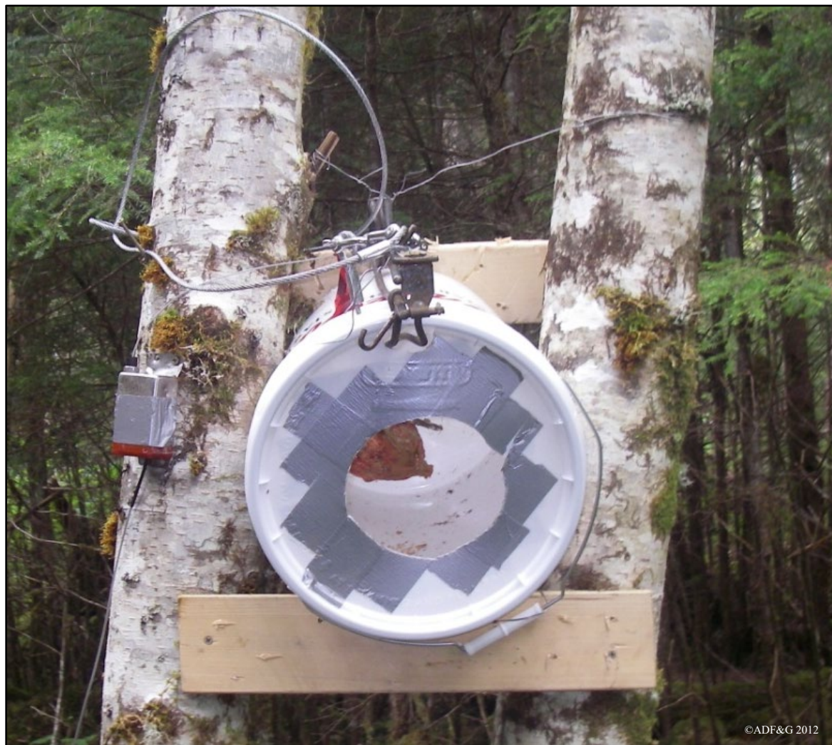
Figure 3. Bucket cable trap fully deployed and operational.
