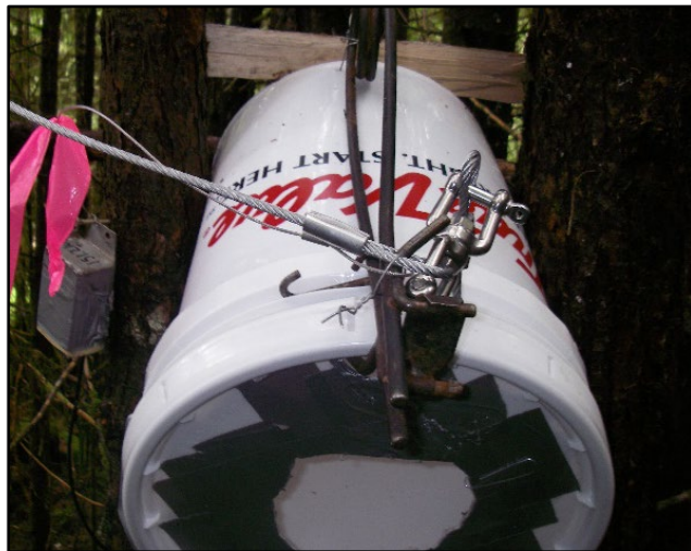
Figure 7. Snare cable attachment to thrower arm.
