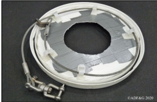
Figure 6. Self-adhesive cable clamps inside bucket lid holding snare cable.
