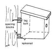
Attach the nest box to a post, tree, or house using a lag bolt and spike nail. The spacing blocks will allow you to open the box easily.
