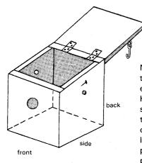
Nail the box together so that the bottom board is enclosed by the four sides. Hinge the roof on one side so that it extends beyond the edges of the four sides of the nest box. Place a latch on the roof so predators won't be able to pry the box open.
