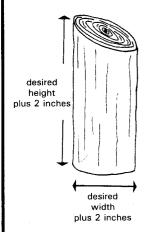
Use a section of birch, aspen, or spruce log from your firewood pile. Be sure to select a log large enough for the inside cavity dimensions required by the bird that will use the house. Cut the bottom of the log section off squarely and cut the top at a slight angle to allow a pitched
