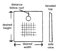
Cut the proper size entrance hole at the correct distance below the top. Roughen the board below the entrance, or attach 1/4-inch mesh screen so that young birds will be able to climb out. Be sure to bevel the top so the roof will fit properly.
