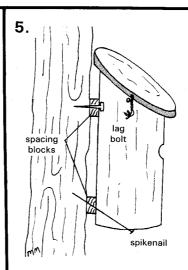
Attach your split log birdhouse to a post or tree using a lag bolt and spike nail. Spacing blocks will allow you to open the lid easily.
