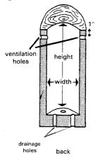
Hollow out the inside of the two halves to the required dimensions using a chisel or chainsaw. Leave the bottom of the log halves solid, but hollow out the top completely. Drill three, 1/8-inch drainage holes through the floor of the back half. Drill 1/8-inch ventilation holes through each side of the back half, 1 inch below the top.
