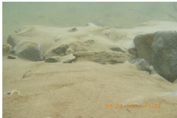
Figure 6.—Sediment from in stream work on substrate.
