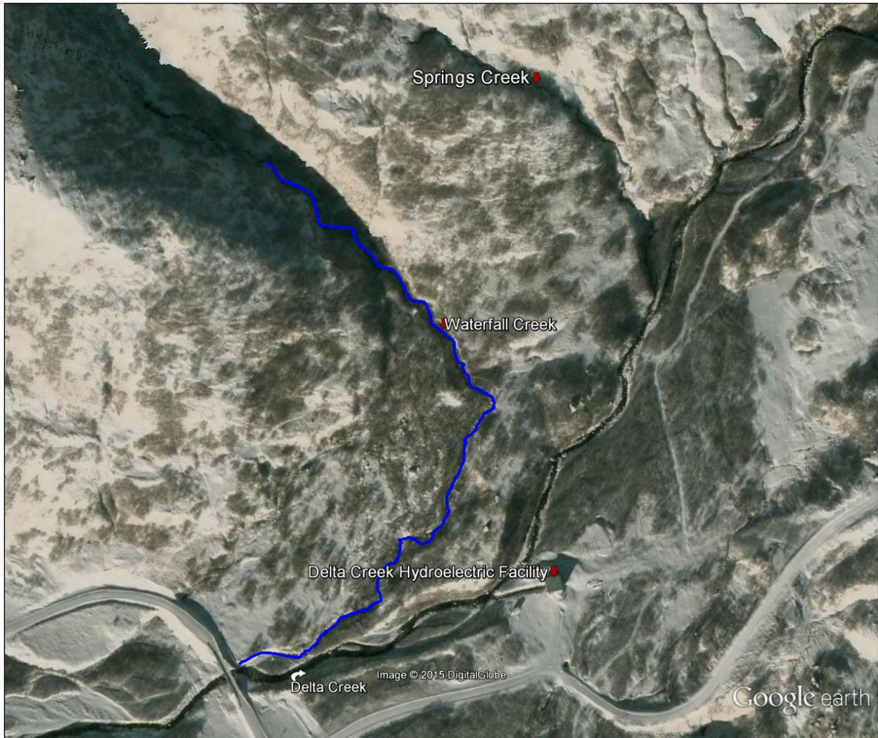
Figure 1.—Waterfall Creek basin and study area. Note the existing Delta Creek Hydroelectric Facility and tailrace, where diverted Waterfall Creek water would be discharged.
