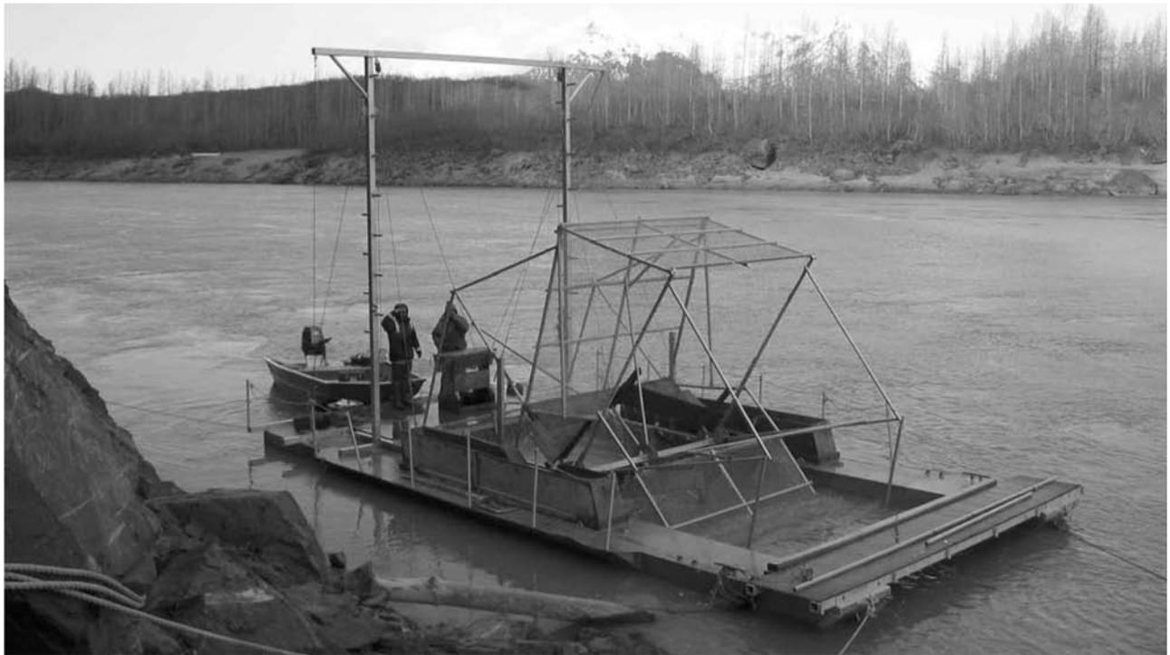
Figure 2. One of the 3 large aluminum fishwheels operated on the Copper River from 2001 to 2004. This photo is of the east-bank fishwheel at Baird Canyon looking southwest and downstream at low water conditions in May 2003.
