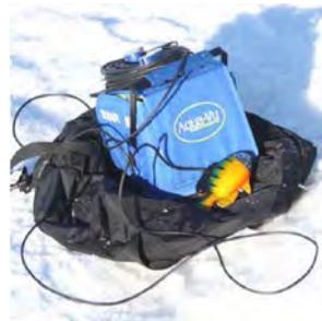
*Portable underwater video cameras allow ice fishers to see if fish activity is occurring around their baits and lures.*
